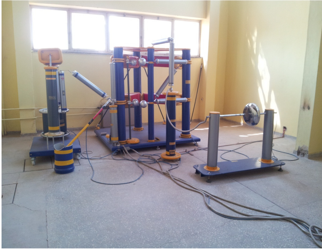
Figure 3. 2 Impulse generator used in the experiments and rod-plane test gap.
