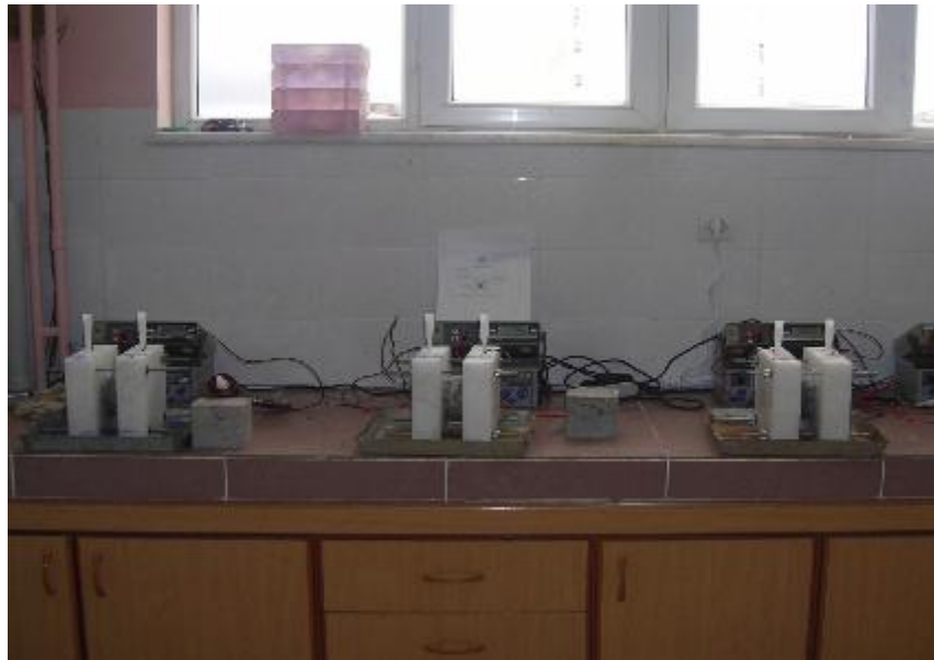
Figure 3.7 Rapid chloride permeability test
