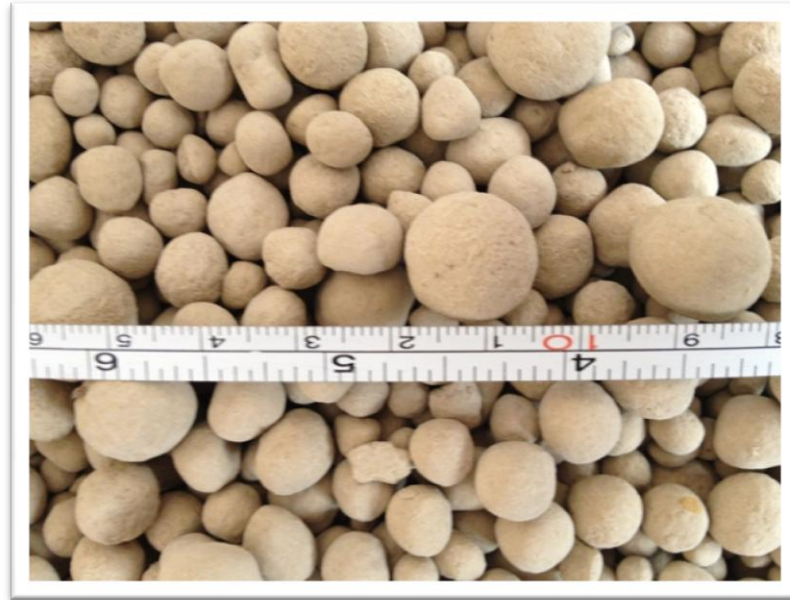
Figure 3.2 View of Cold bonded slag aggregate
