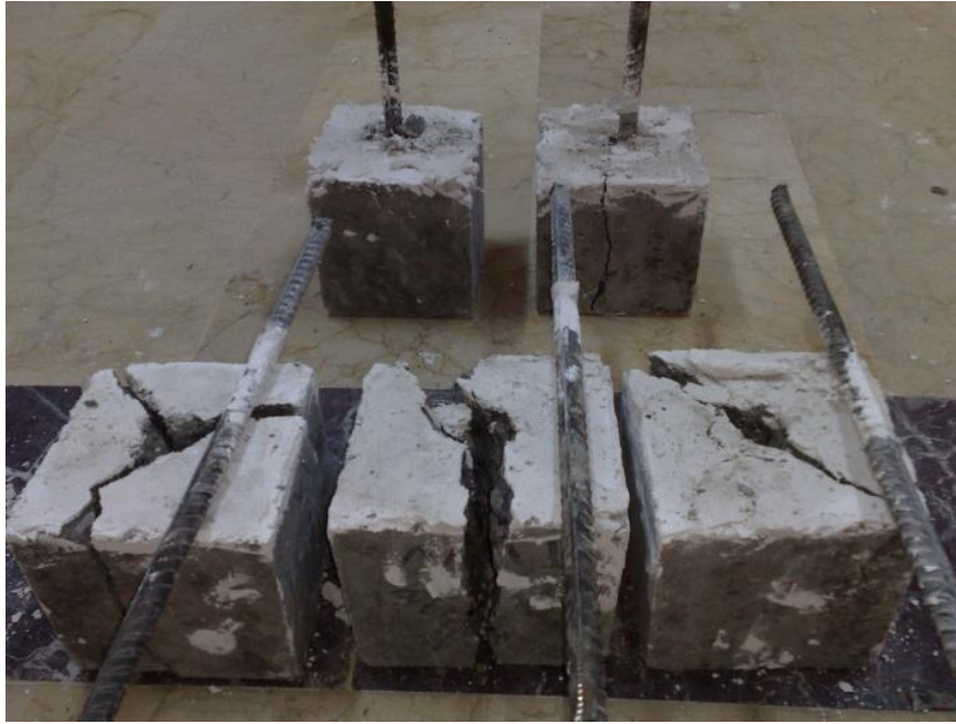
Figure A13 Photographic view of pullout specimens (splitting failure)
