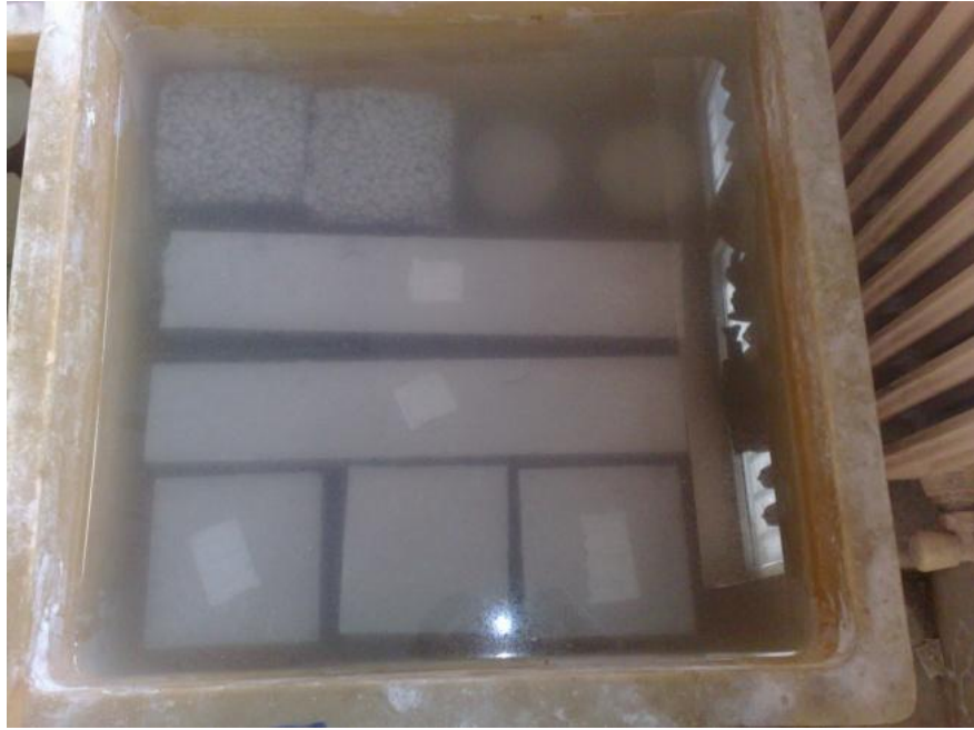
Figure A9 Photographic view of the samples during curing
