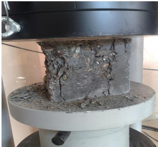
Figure A14 Photographic view of compressive strength specimens
