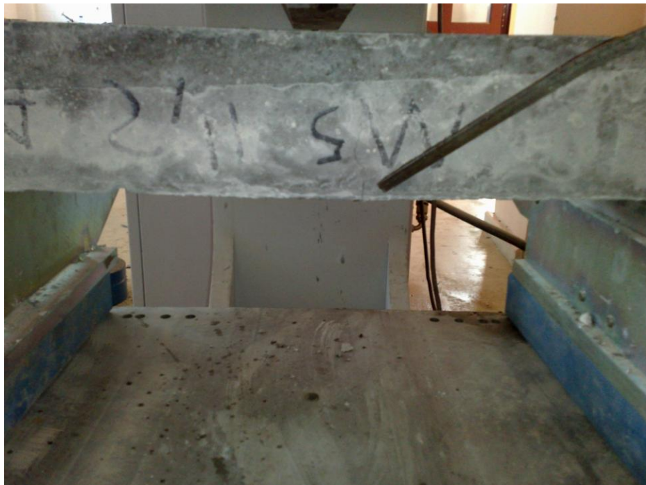
Figure A10 Photographic view of three point flexural testing
