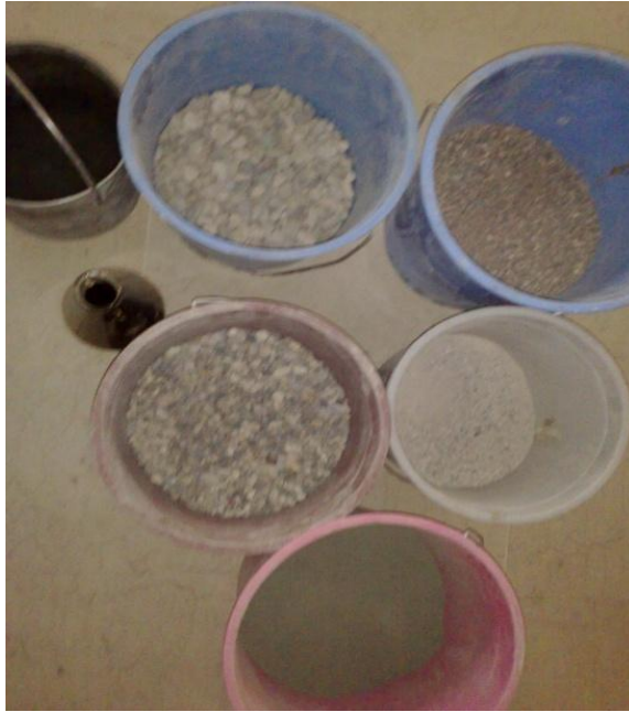
Figure A1 Photographic view of used materials (Portland cement, aggregate, Super plasticizer, water).
