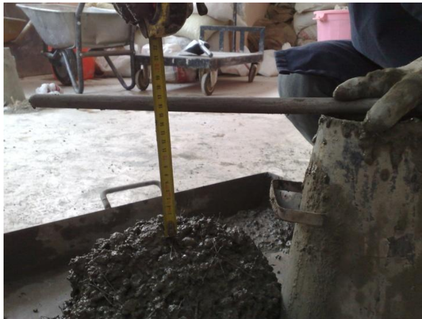
Figure A4 Photographic view of slump test-1
