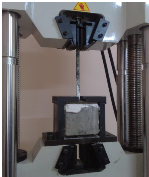
Figure A12 Photographic view of bond strength specimens and pull out device
