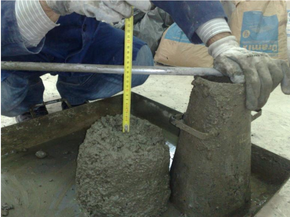
Figure A5 Photographic view of slump test-2
