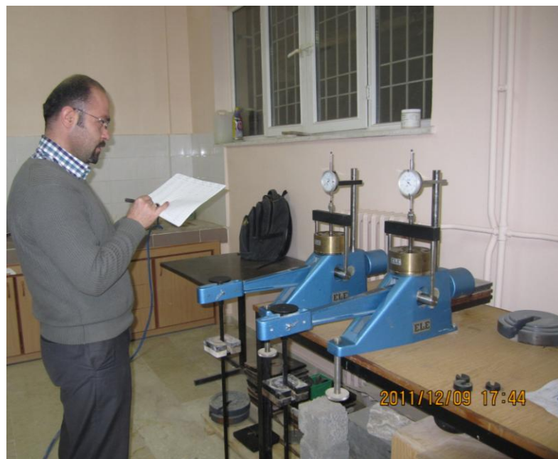
Figure 4.5 Oedometer testing machines used during the experimental works
