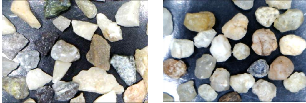
Figure 4.1. Pictures of (a) Crushed stone sand, and (b) Trakya sand used during the experimental study
