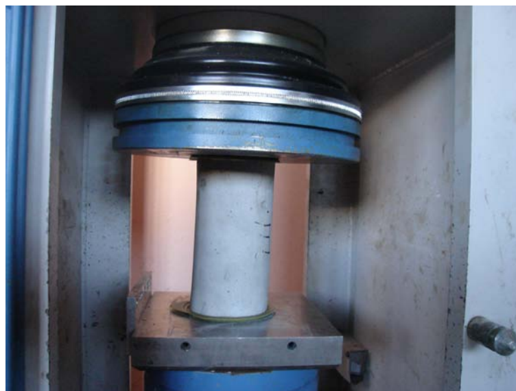
Figure 3.7 Compression testing machine with a cylinder sample
