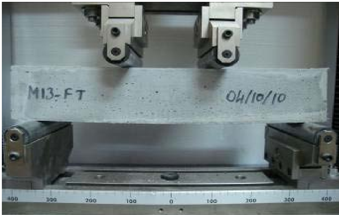
Figure 3.8 Four-point bending test
