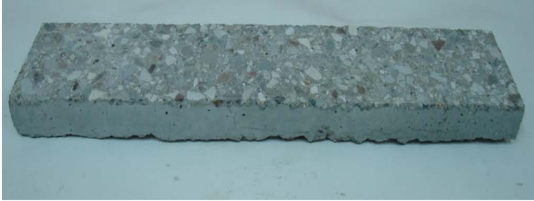
Figure 3.12 Substrate specimen with 30 mm thickness after diamond saw cutting
