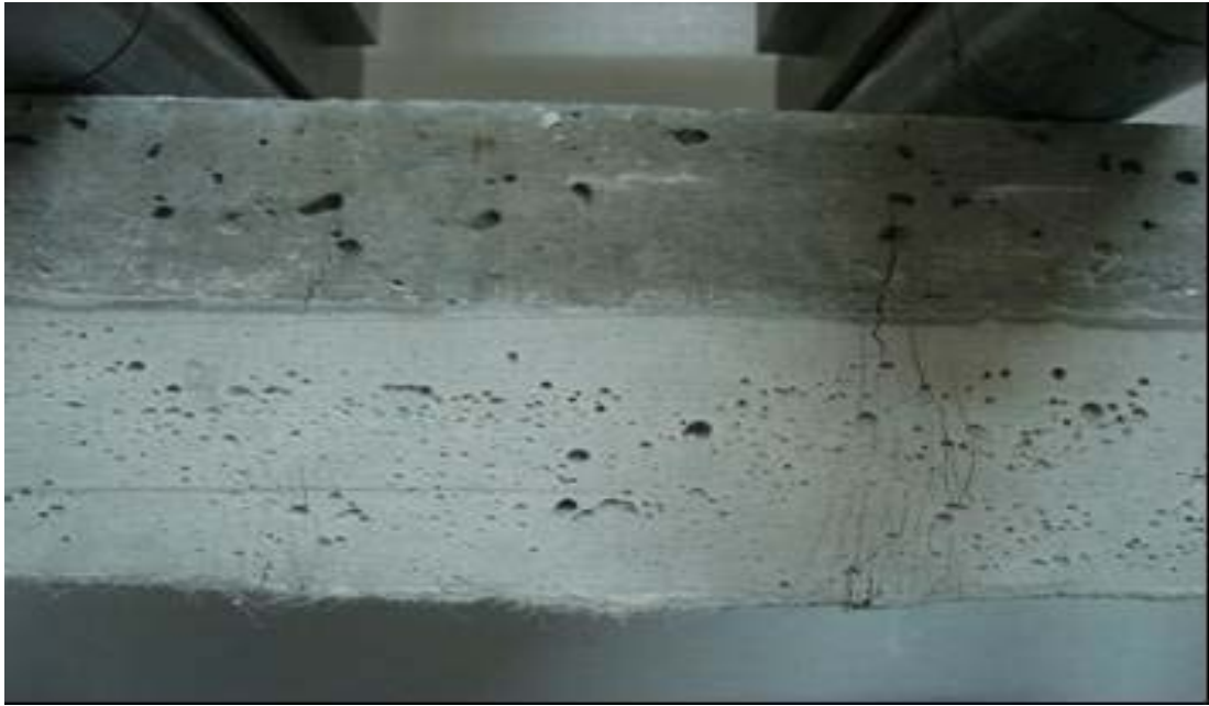
(b) S_ECC composite beam after four point bending test
