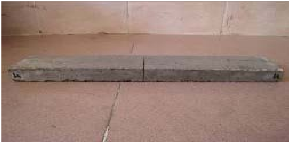
Figure 3.14 Substrate specimen after cutting (30 mm thickness) with a vertical crack
