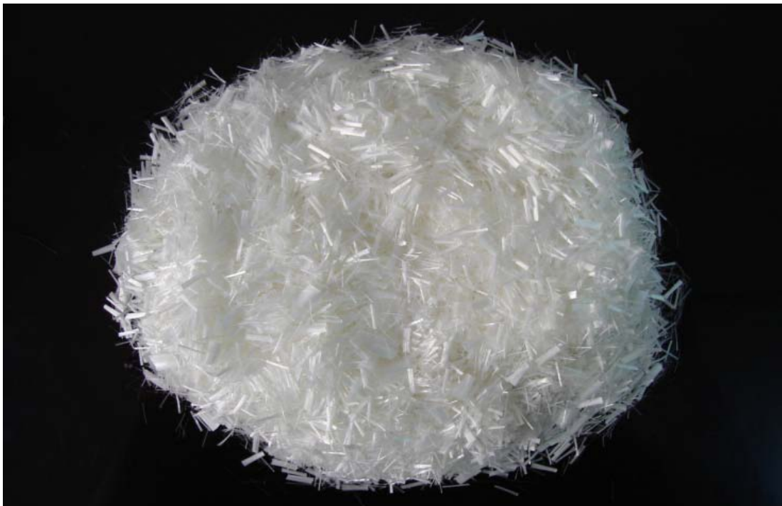
Figure 3.4 PVA Fiber used in the production of ECC
