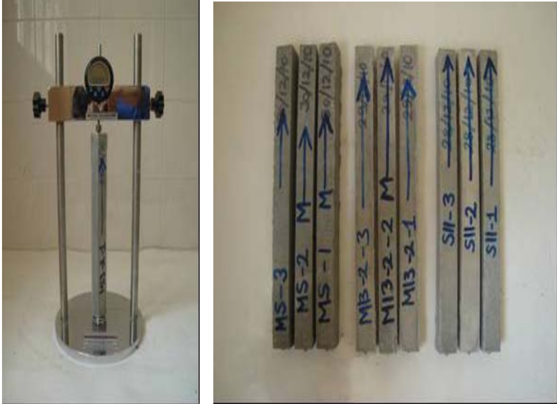
Figure 3.10 Drying shrinkage device and samples
