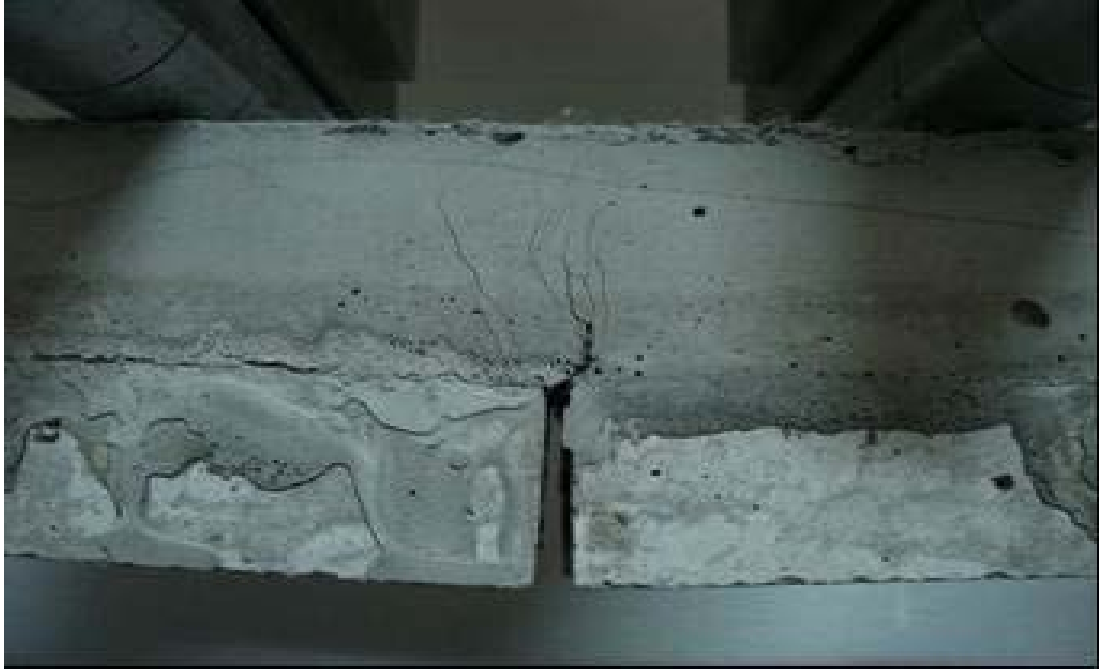
(b) F_ECC composite beam
