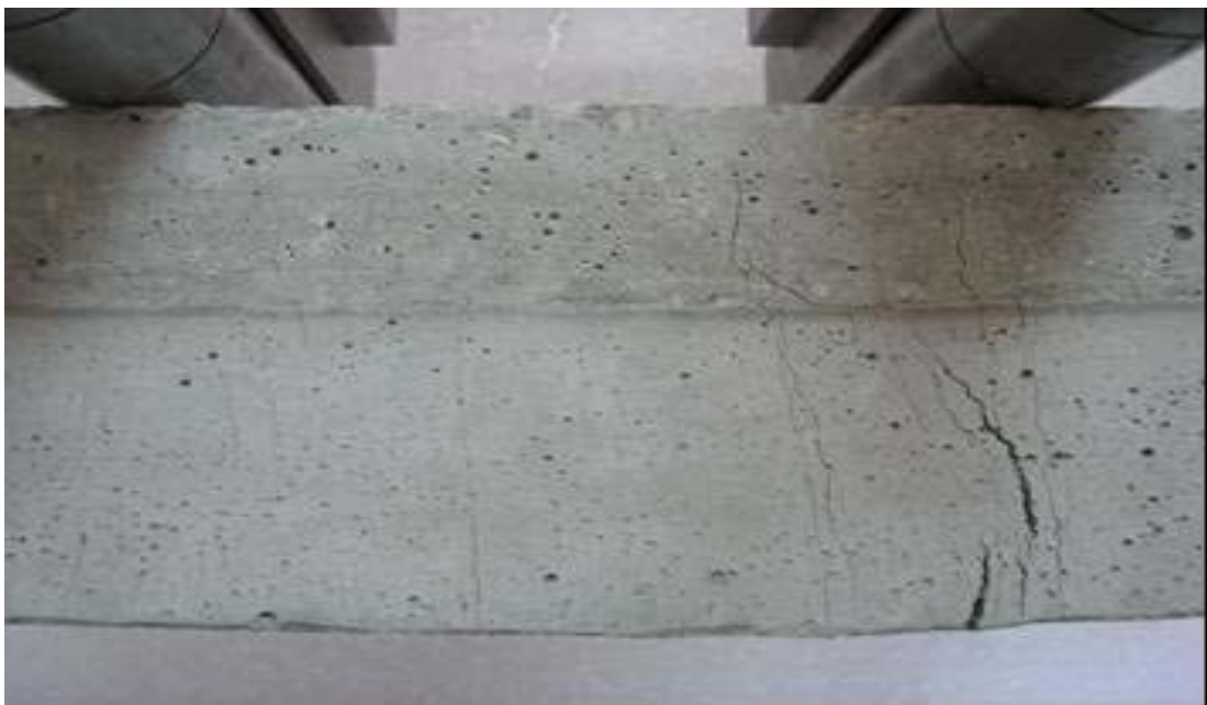
(c) F_ECC composite beam after four point bending test
