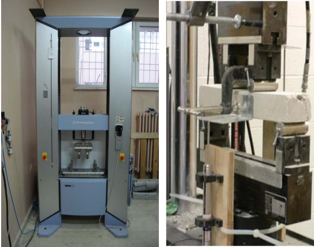
Figure 3.9. Four-point flexural strength test
