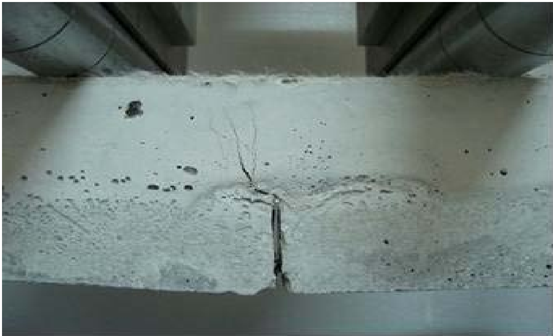
(a) S_ECC composite beam
