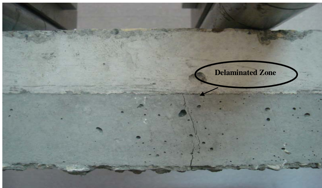
(a) MSC composite beam after four point bending test
