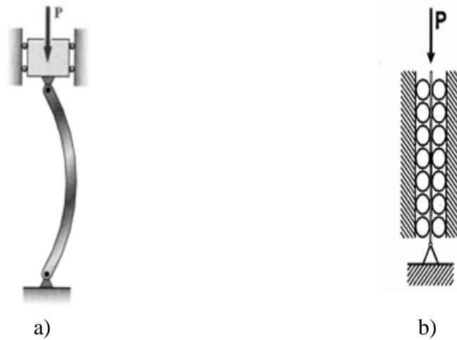
Figure 2.8 Schematic diagram of a) conventional brace and b) buckling restrained brace
