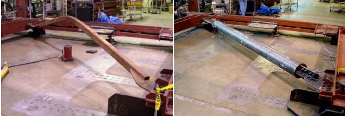
a) Behavior of conventional brace and buckling restrained brace tested in laboratory
