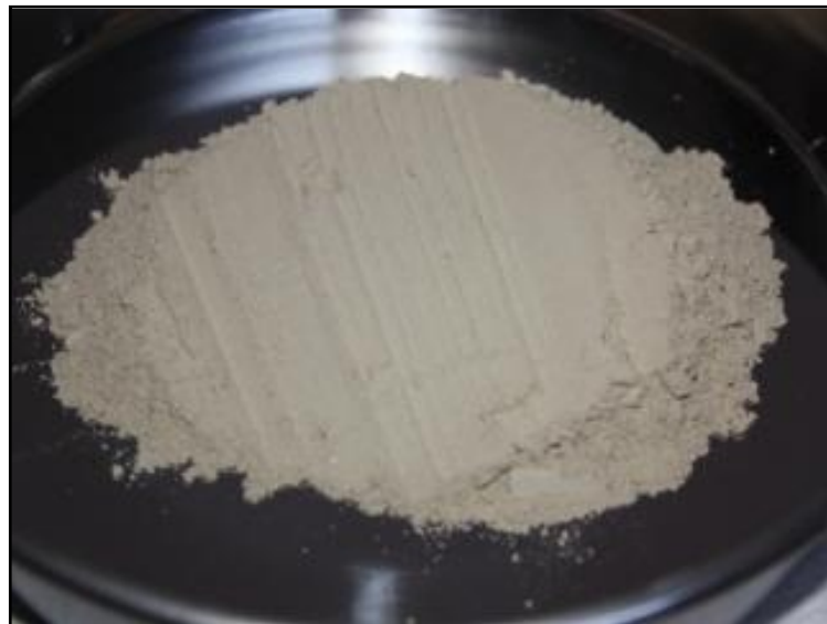
Figure 4.4 Rice husk after grounding (RHP)
