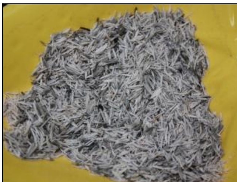
Figure 4.5 Rice husk after burning at 600C°(RHA)
