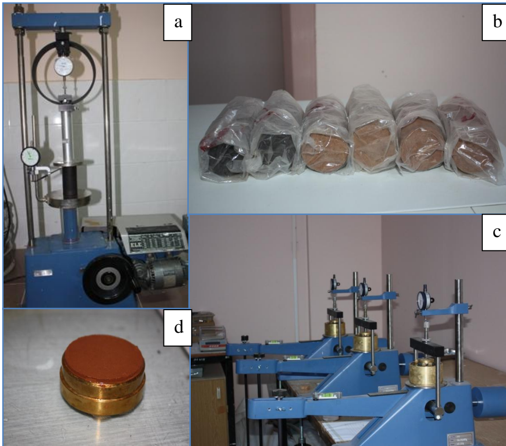
Figure 4.8 (a) unconfined compressive strength- UCS device, (b)UCS specimens, (C) Oedometer device and (d) specimen after swelling test
