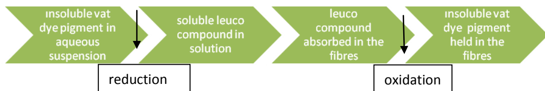
Figure 4.4: Indigo dyeing steps
