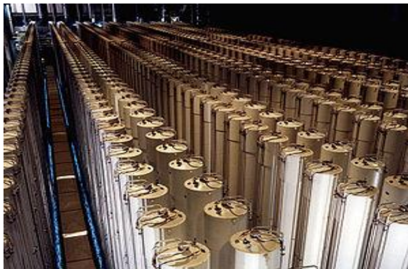
Figure 3.3 Gas centrifuge cascade [40].
