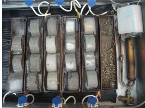
Figure 3.11 Specimens in freezing and thawing machine
