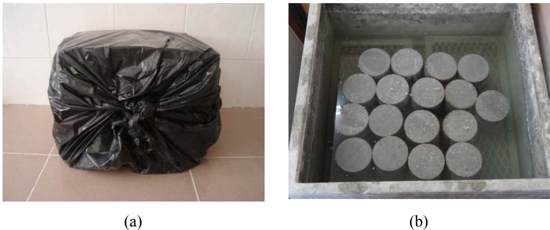
Figure 3.5 Curing of ECC specimens after production of them (a) Cube and prism specimens, (b) Cylindrical specimens
