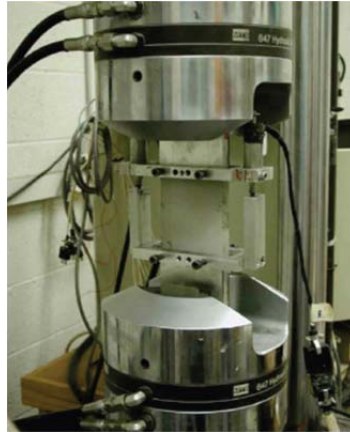
Figure 2.8 Uniaxial tensile test set up
