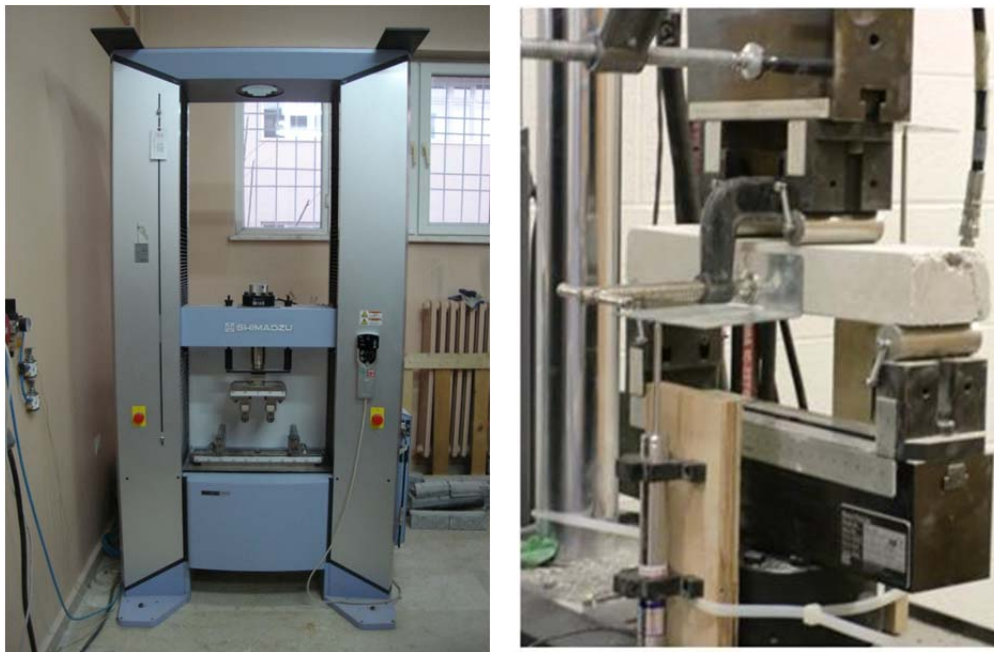
Figure 3.10 Four-point flexural strength test
