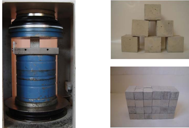
Figure 3.8 Compression testing machine and cubic samples
