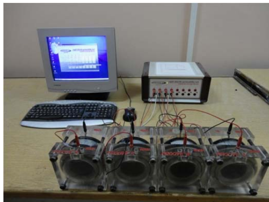
Figure 3.12 Rapid chloride permeability test (RCPT) setup
