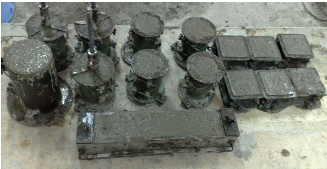
Figure A.6 Test specimens after mixing, vibrating, and finishing
