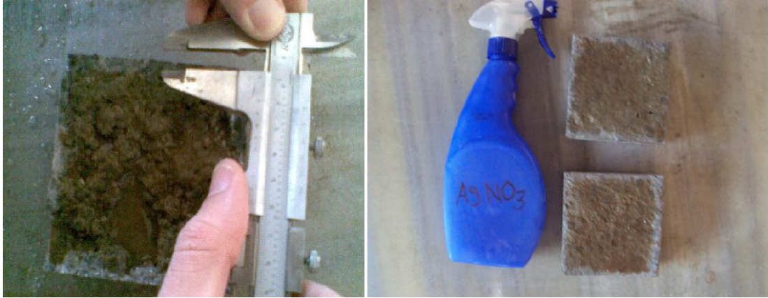
Figure A. 9 Measurement of salt penetration
