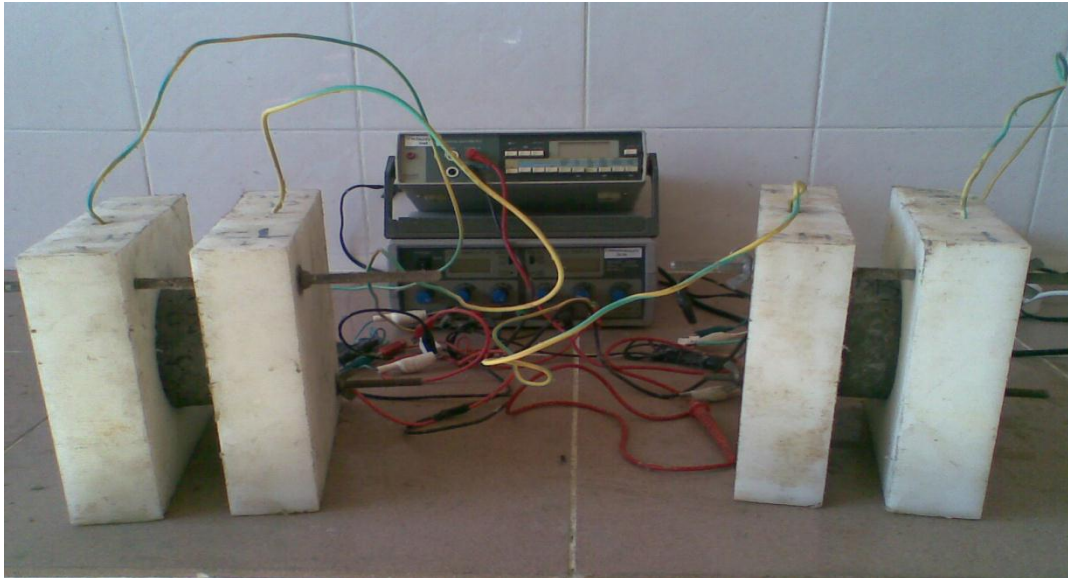
Figure A.8 RCPT set-up
