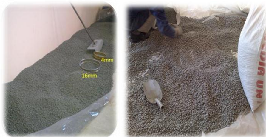
Figure 3.5 Lightweight aggregate stock after 28 days curing
