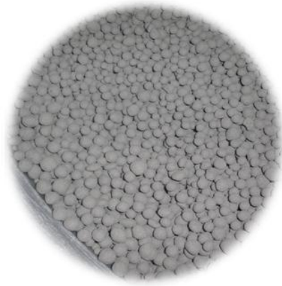
Figure 3.3 Spherical pellets formation after approximately 20 minutes
