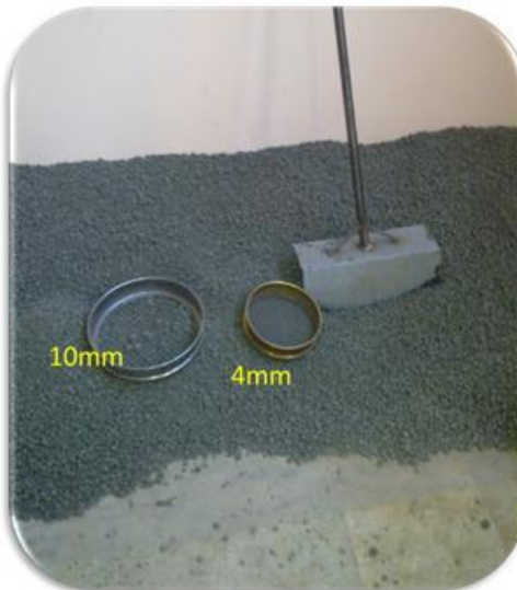
Figure A.4 Hardened lightweight aggregate sieved and ready for mixes
