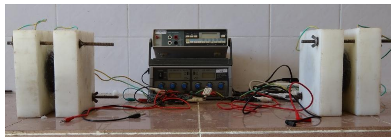
Figure 3.12 Photographic view of the RCPT test set up
