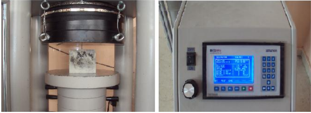
Figure A.7 Measurement of compressive strength
