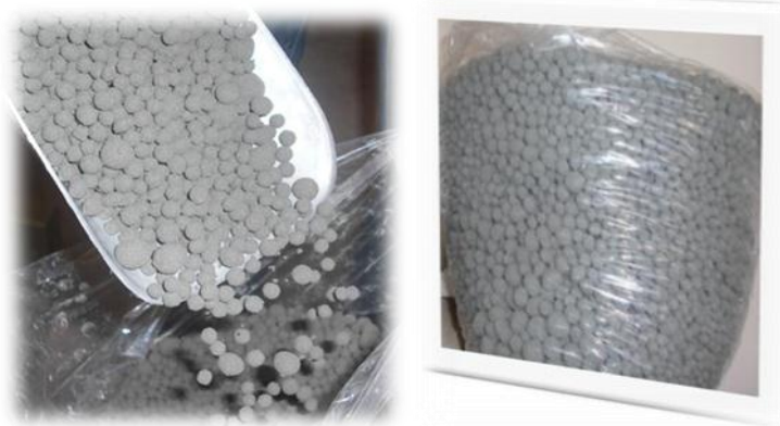
Figure 3.4 Moisture curing of fresh aggregates by keeping in sealed plastic bags
