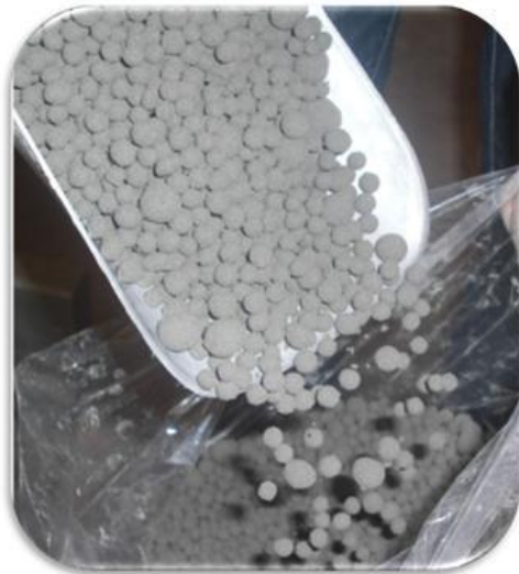
Figure A.3 Fresh lightweight aggregate kept in sealed bags for air curing
