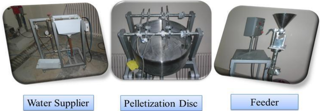
Figure A.1 Photographic view of pelletization system
