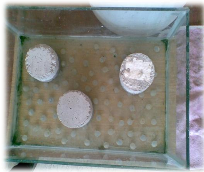
Figure 3.7 View of sorptivity test
