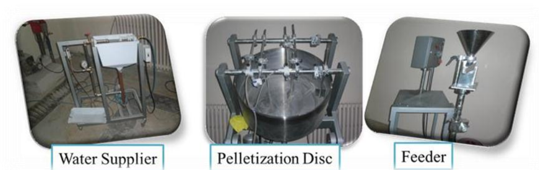
Figure 3.1 General shape of the pelletization disc
