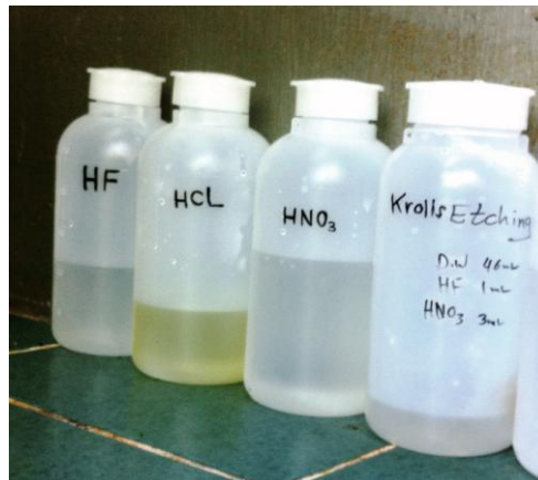
Figure 3.10 Etching solution for Ti-6AL-4V
