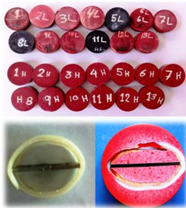
Figure 3.7 Sample specimens mounted in Bakelite
