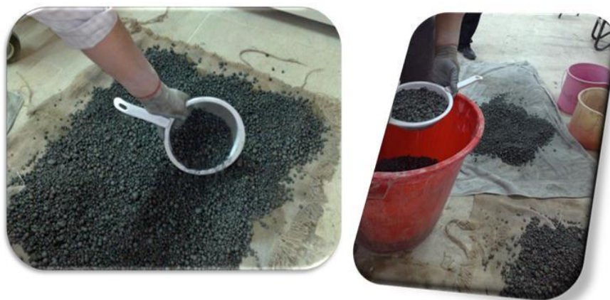
Figure A.5 Immersing aggregate for 30 min in water. to get SSD aggregate
