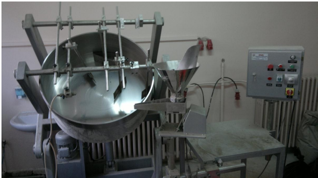
Figure A.2 General views of pelletization disc
