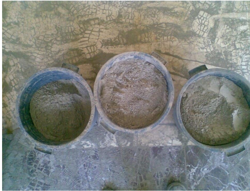
Figure A.1 preparation fly ash and cement to make AFA
