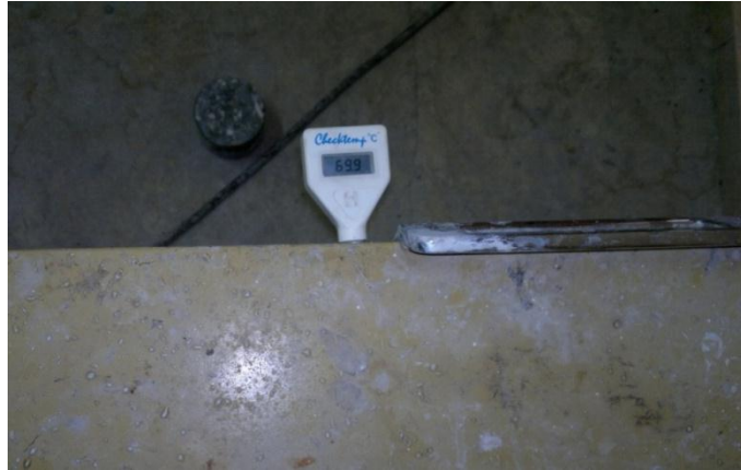
Figure A.10 The required temperature of the steam curing chamber reached
