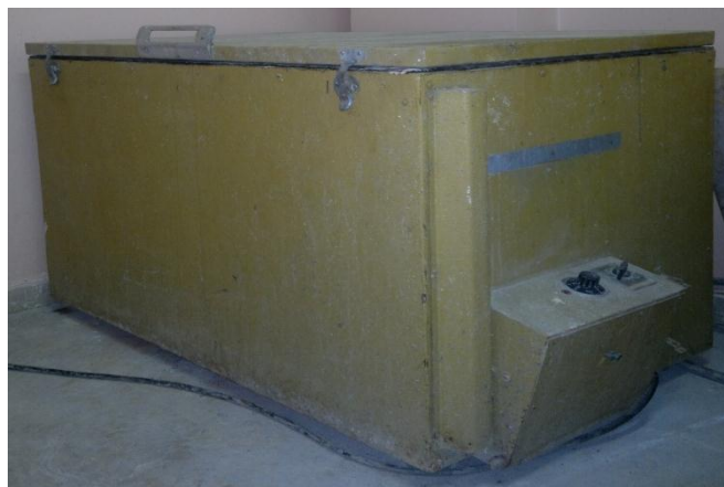
Figure A.12 Photographic view of steam curing chamber
