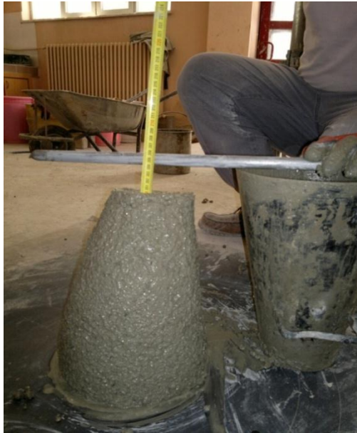
Figure A.8 Photographic view of slump test
