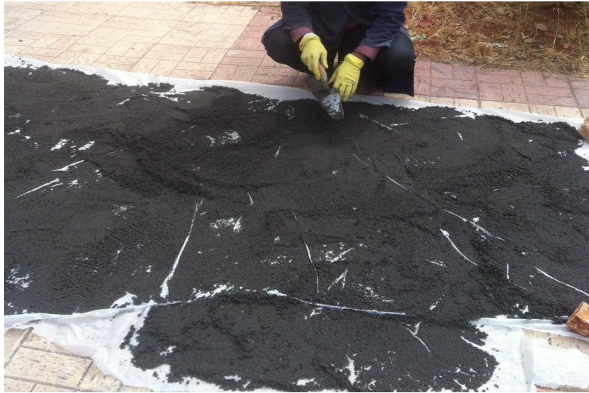
Figure A.6 Immersing aggregate for 30 min in water. To get SSD aggregate
