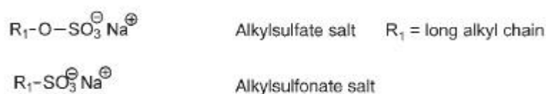
Figure 2.5 Chemical structures of typical anionic softeners [1].
