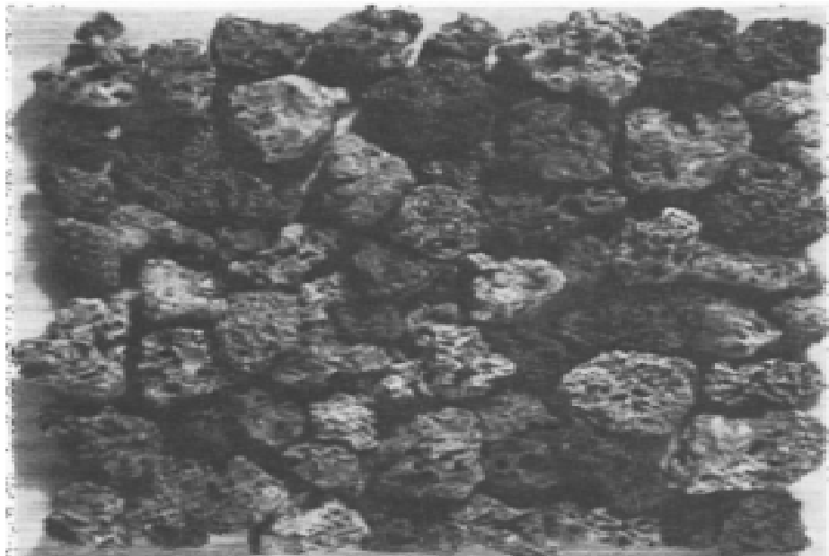
Figure 2.3 Typical foamed slag particles (Newman and Choa, 2003).
