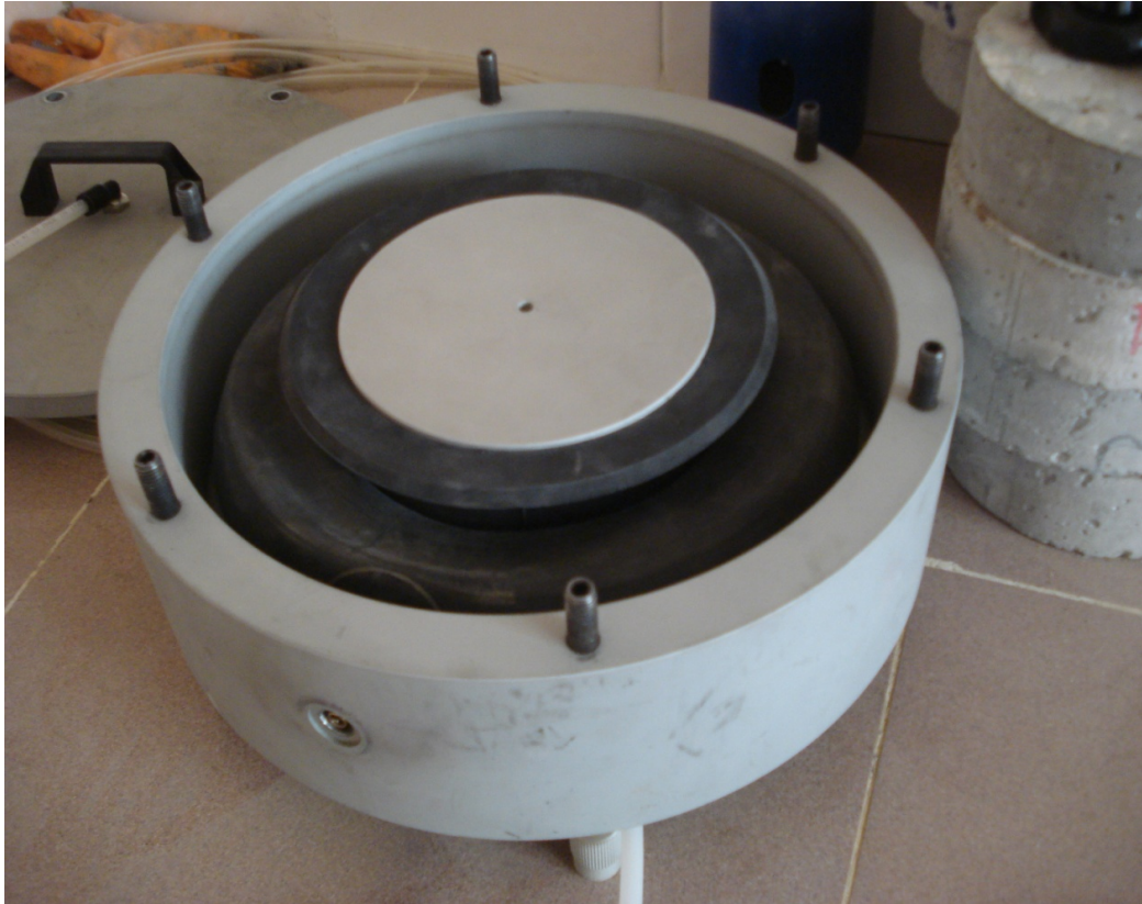
Figure 3.11. Gas permeability test: a) photographic view of the gas permeability set up, b) schematic presentation of set-up, and c) photographic view of pressure cell inside
