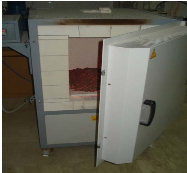
Figure 3.2 Sintered aggregates in muffle furnace
