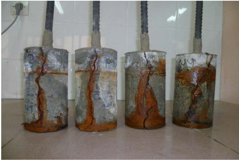
Figure 3.16 Typical cracked samples after accelerated corrosion test
