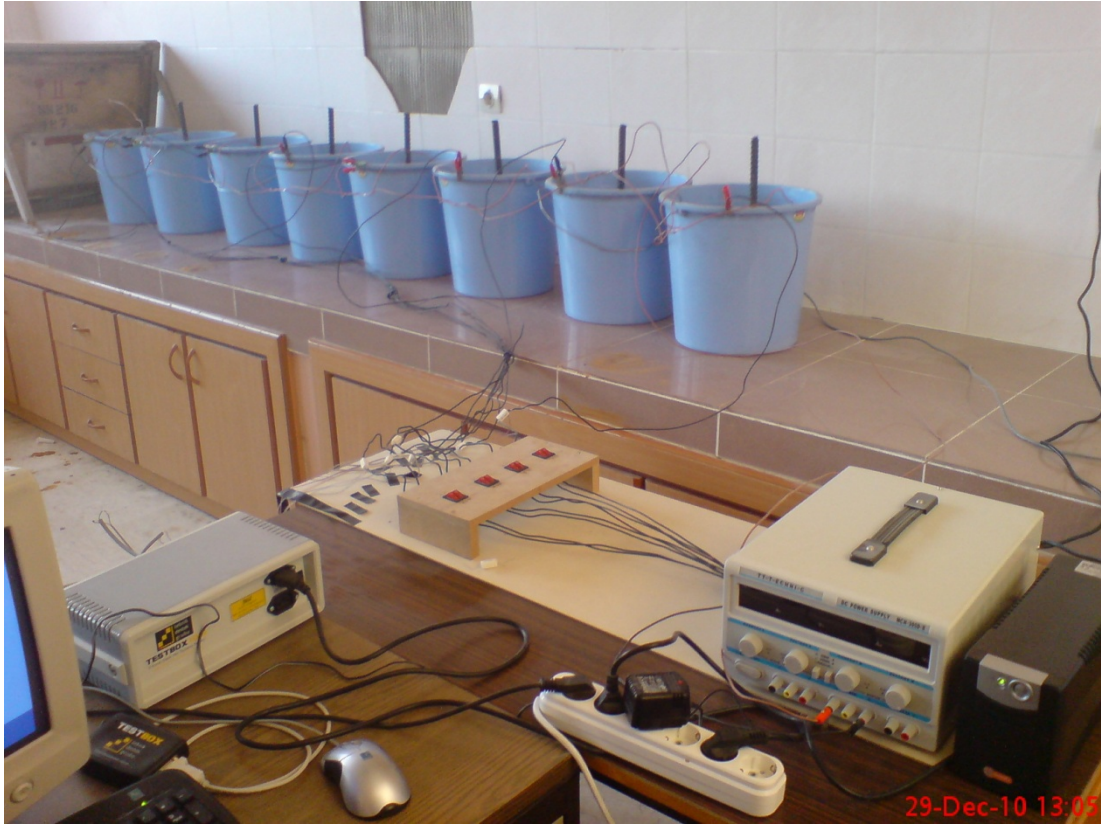
Figure 3.14 Photographic view of the accelerated corrosion test set up
