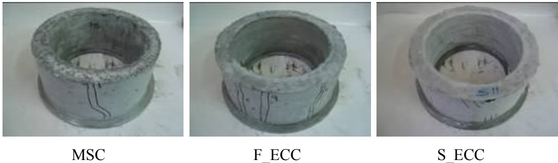
Figure 3.22 Restraining ring shrinkage samples of overlay mixtures
