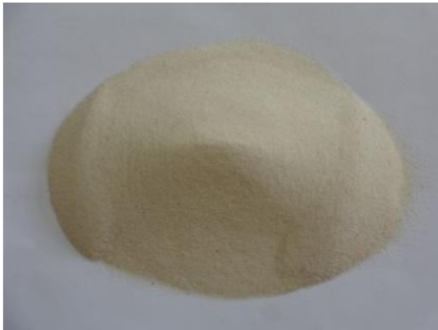
Figure 3.4 Fine quartz sand used in the production of ECC
