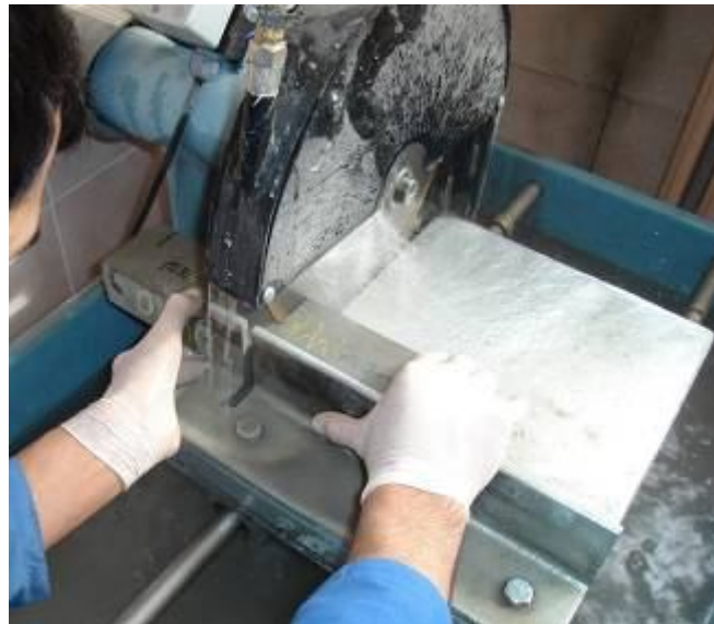
Figure 3.10 Notch opening of a specimen for determining fracture toughness
