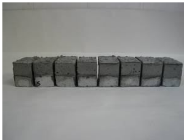
Figure 3.34 Final view of splitting prism test samples
