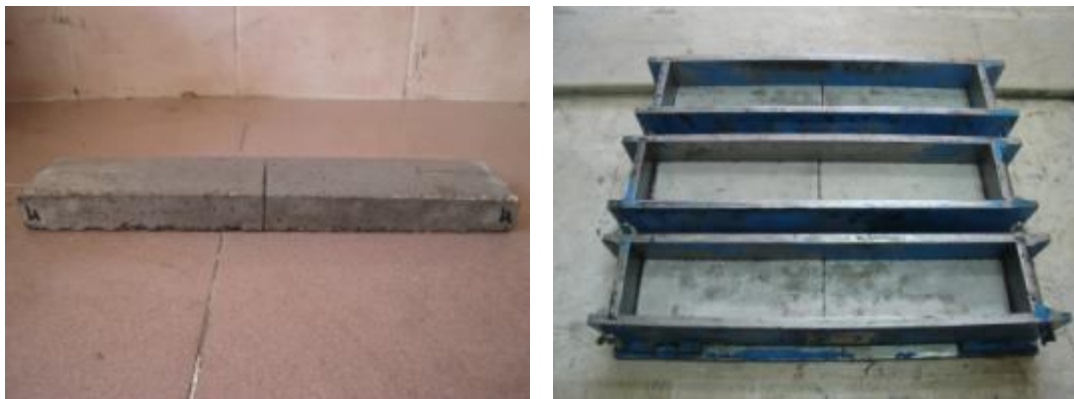
Figure 3.28 SUBC sample preparation for reflective cracking test
