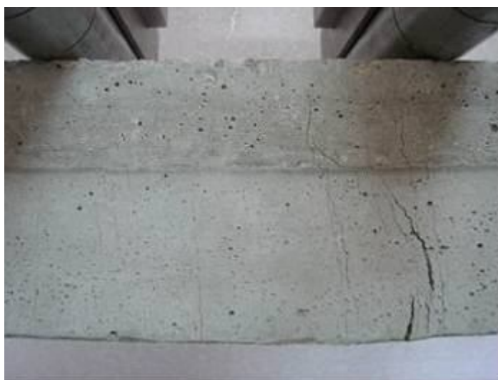
c) F_ECC composite beam after four point bending test
