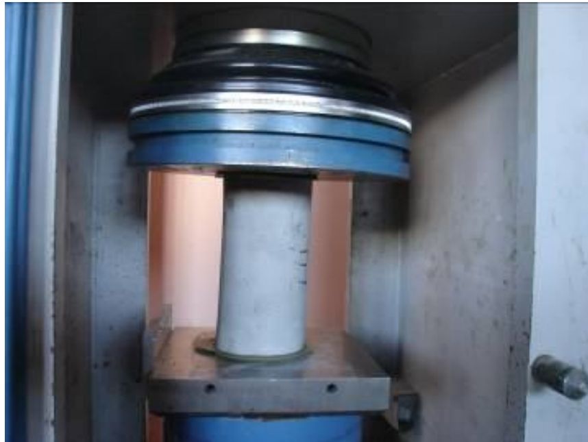
Figure 3.19 Compressive strength testing machine with a cylinder sample
