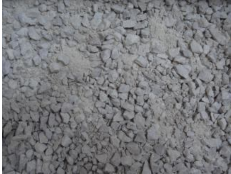
Figure 3.17 Combined aggregate used in the production of SUBC and MSC
