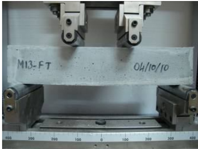
Figure 3.20 Four-point bending test
