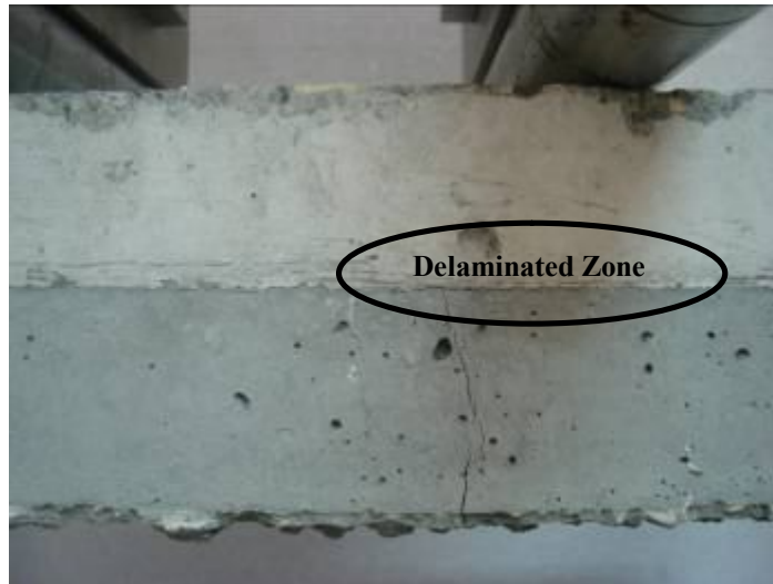
a) MSC composite beam after four point bending test
