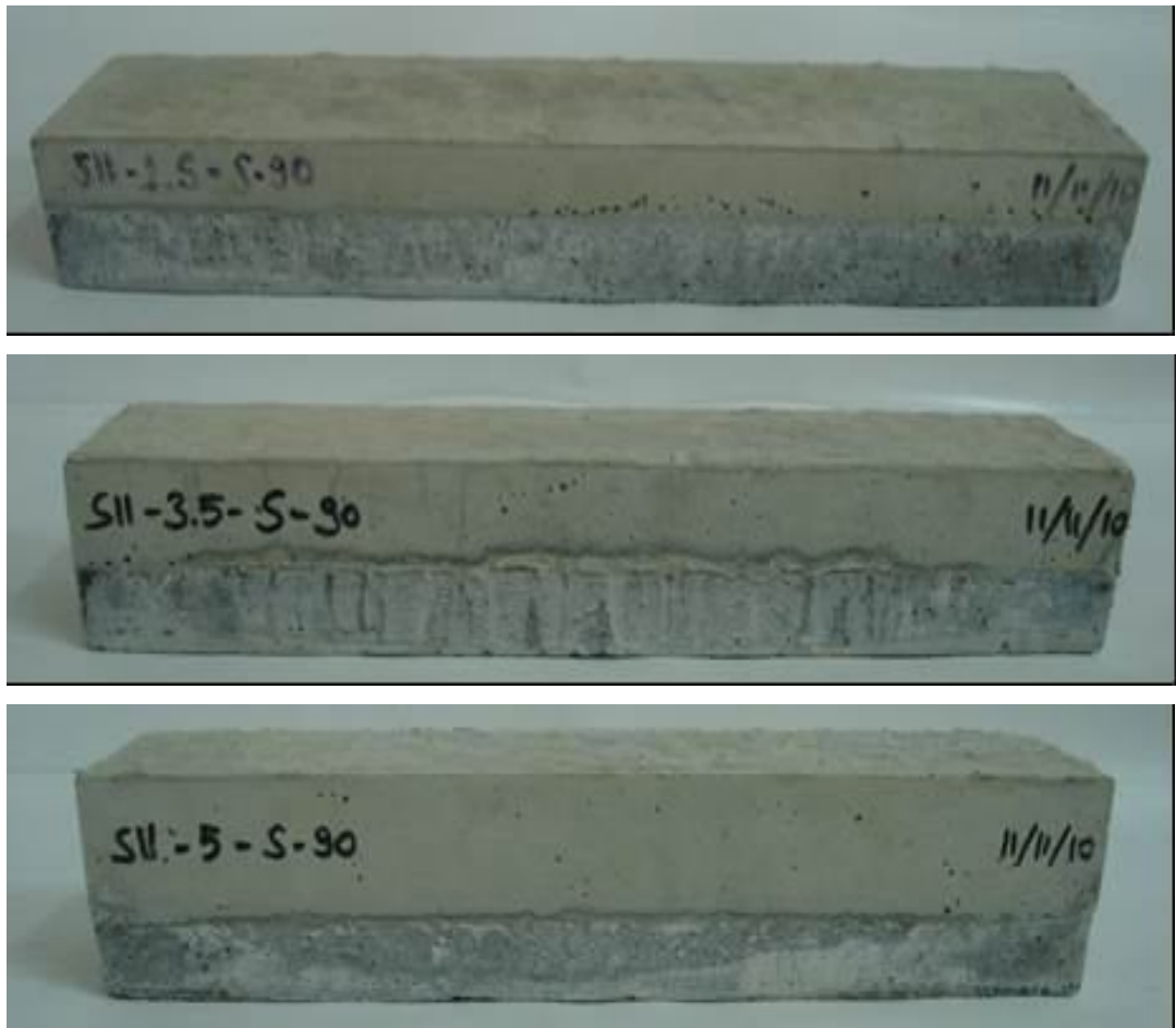
Figure 3.26 Layered specimens with different thicknesses for flexural performance
