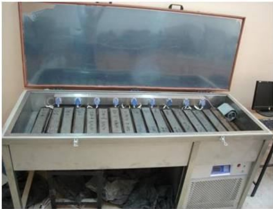
Figure 3.16 Freezing and thawing test
