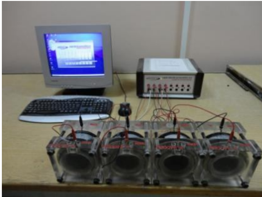
Figure 3.23 Rapid chloride permeability test set-up
