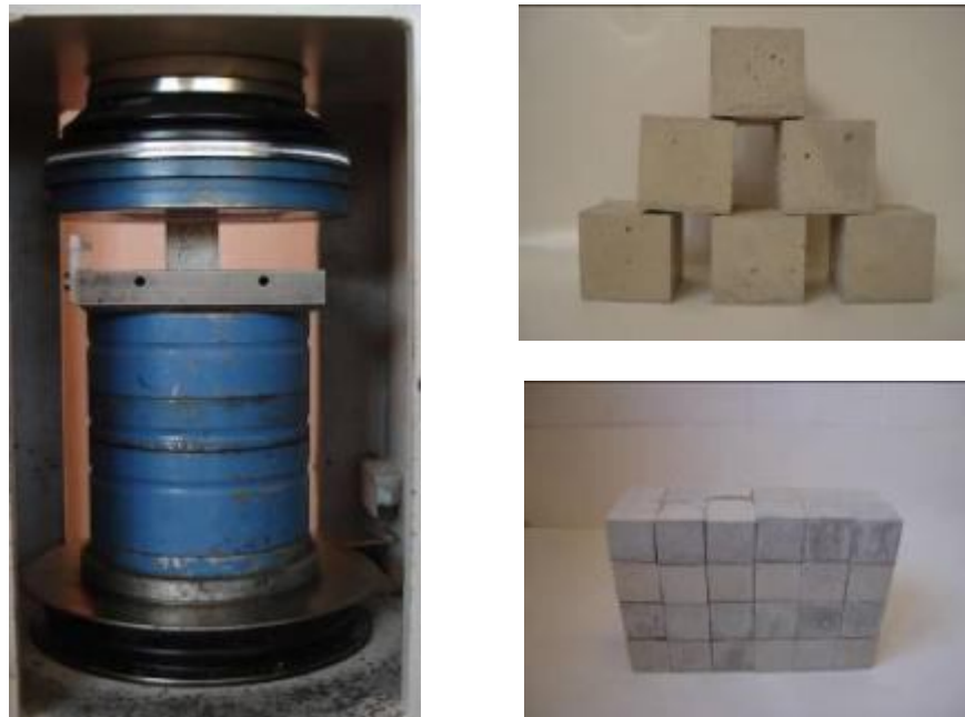
Figure 3.8 Compression testing machine and cubic ECC samples
