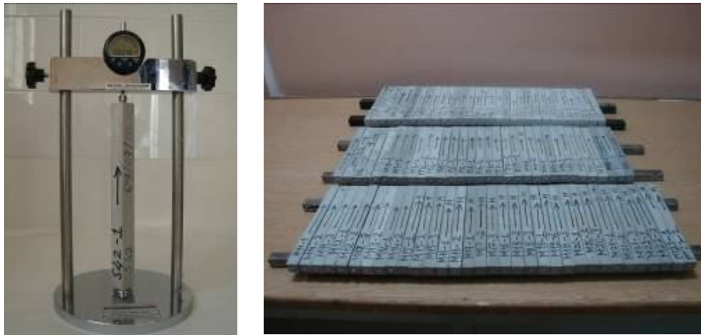
Figure 3.14 Drying shrinkage device and samples
