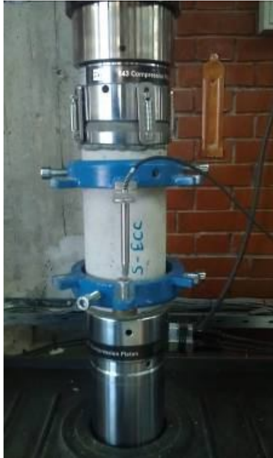
Figure 3.25 Experimental test set-up of modulus of elasticity
