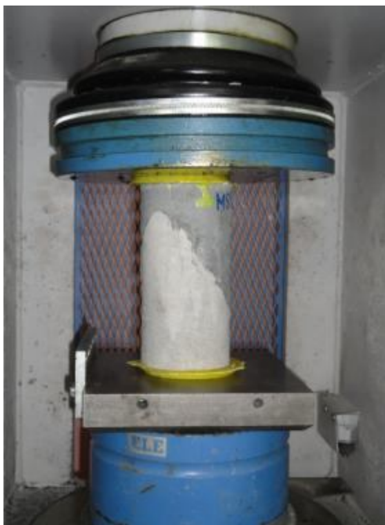
Figure 3.31 Slant shear test set-up
