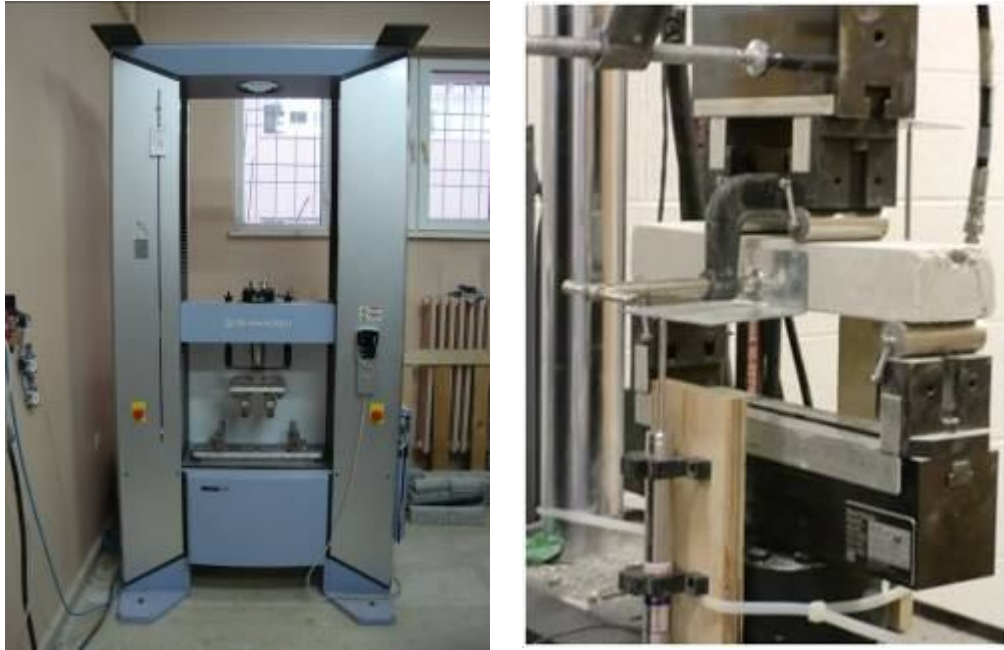
Figure 3.12 Four-point flexural strength test
