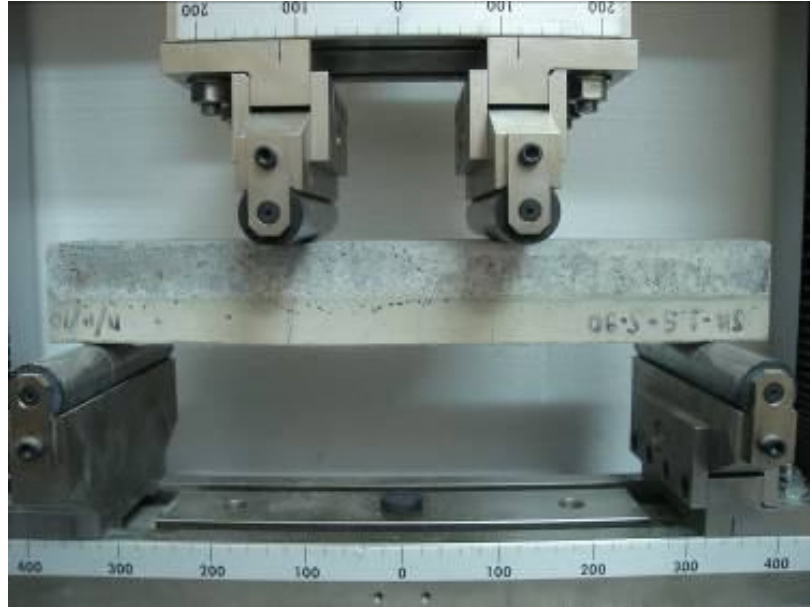
Figure 3.27 Four-point bending test of overlaid specimen
