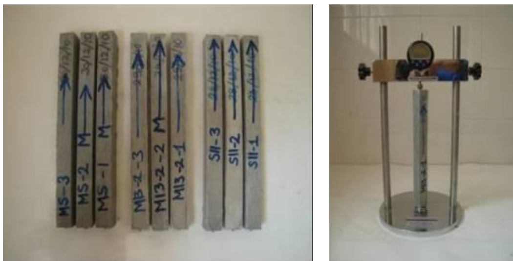
Figure 3.21 Drying shrinkage samples of overlay mixtures and device
