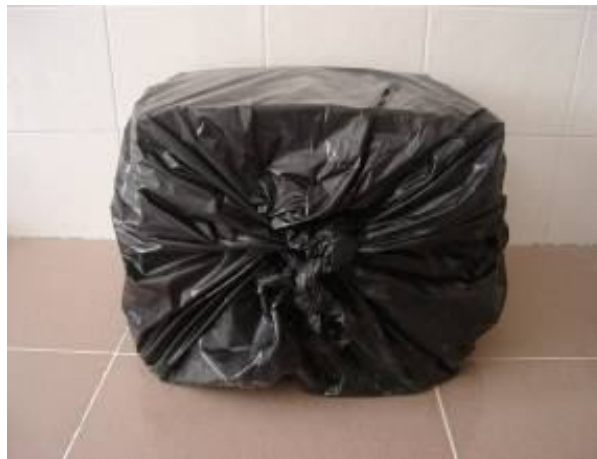
Figure 3.7 Curing of ECC specimens under sealed condition
