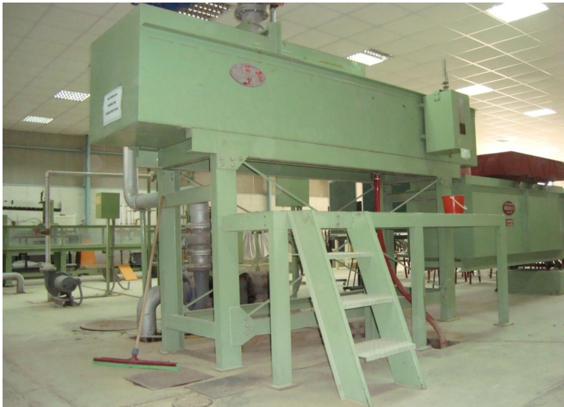
Figure 4.3 The Overhead tank and the V-notch weir used in the study
