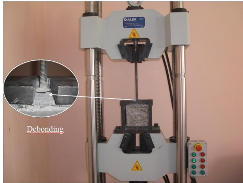
Figure 3.14 Photographic view of the pullout test set up during testing the specimen
