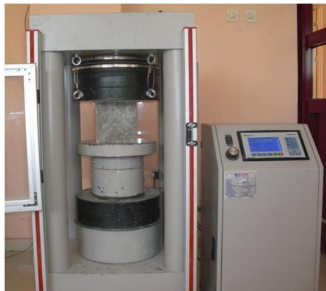
Figure 3.9 Compressive strength test machine with 2000 kN capacity
