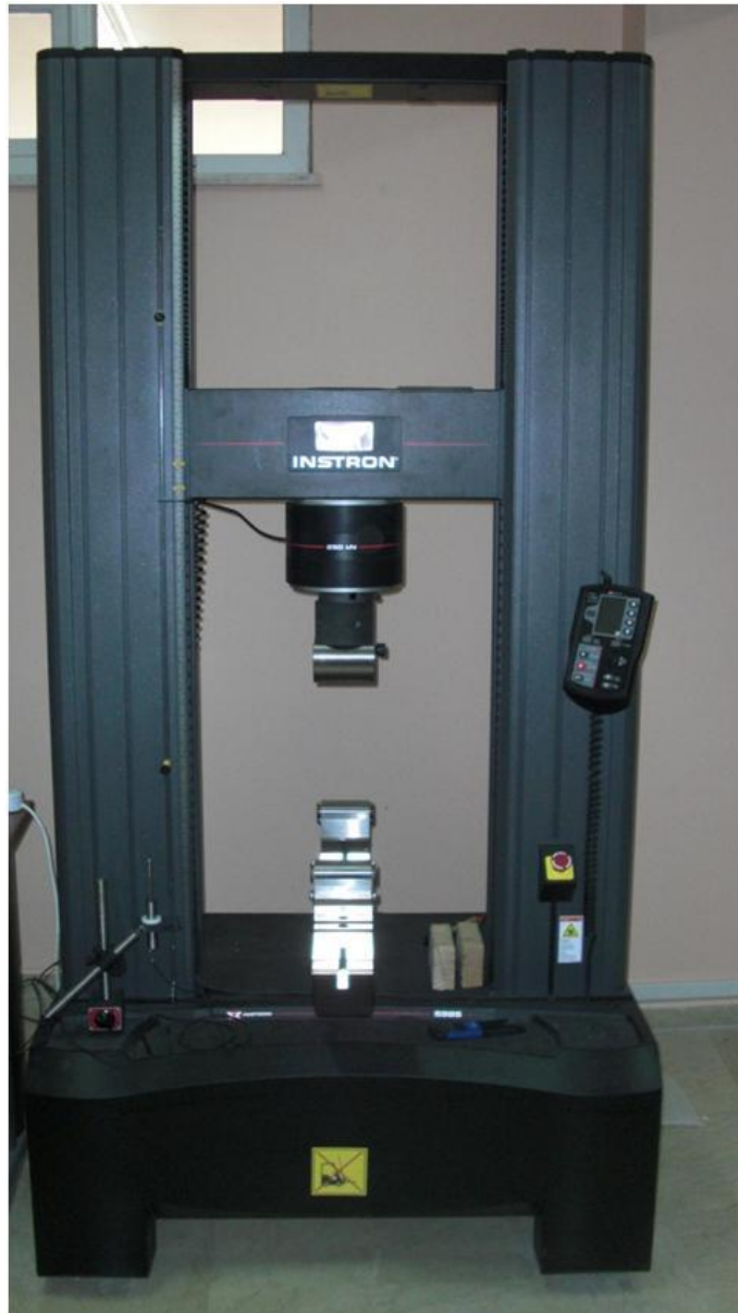
Figure 3.11 Universal testing devices and three point flexural testing fixture
