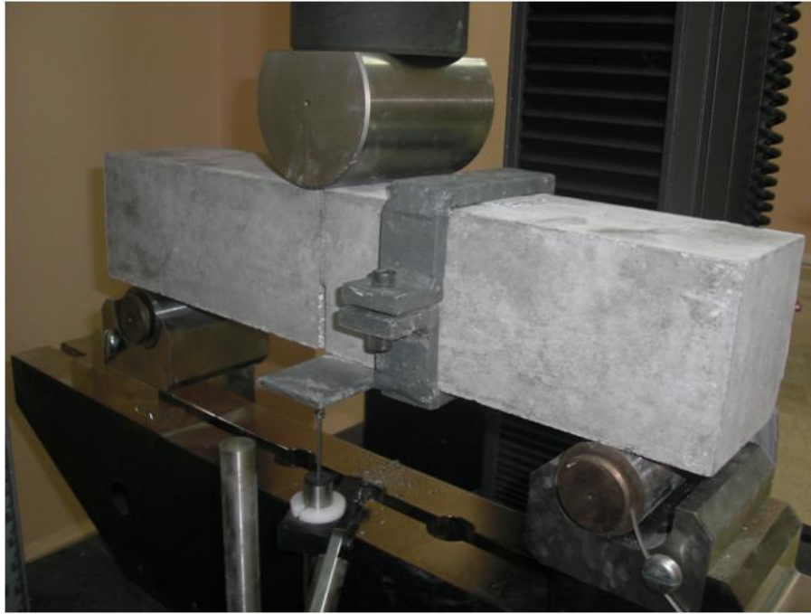
Figure 4.5 Photographic view of: a) notched beam and b) subjected to three-point bending test
