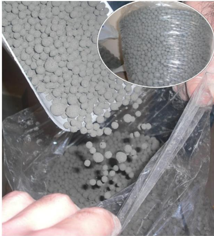
Figure 3.3 Keeping the aggregate in sealed plastic bags
