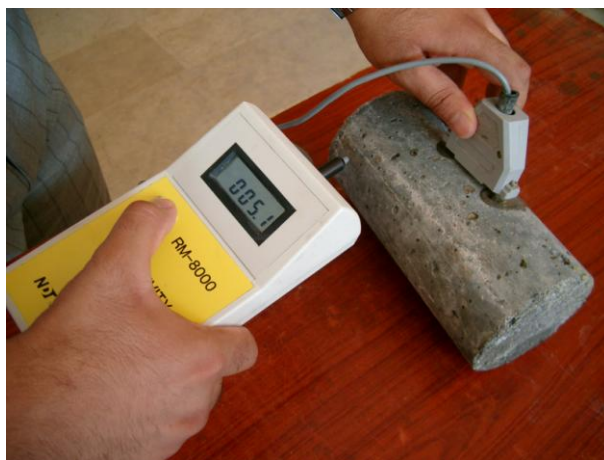
Figure 3.10 Photographic view of the ER test device
