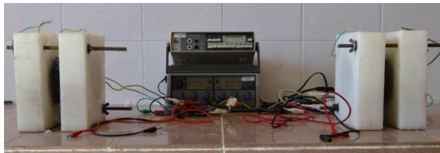
Figure 3.6 Photographic view of the RCPT test set up
