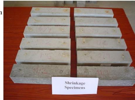
Figure 3.16 Free shrinkage specimens
