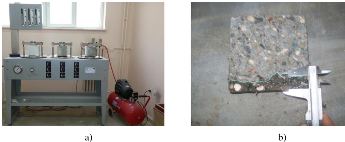
Figure 3.7 Water permeability test: a) device and b) measurement of penetration depth
