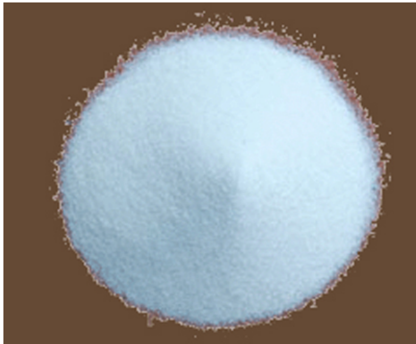
Figure 3.2 A view of quartz sand aggregate
