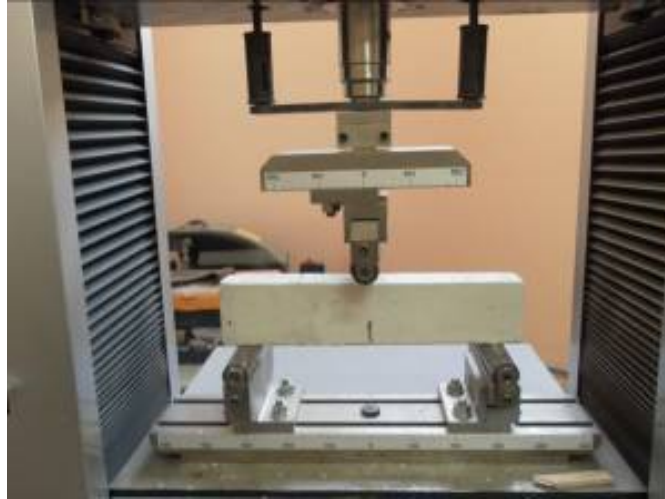
Figure 3.11 Fracture toughness test setup
