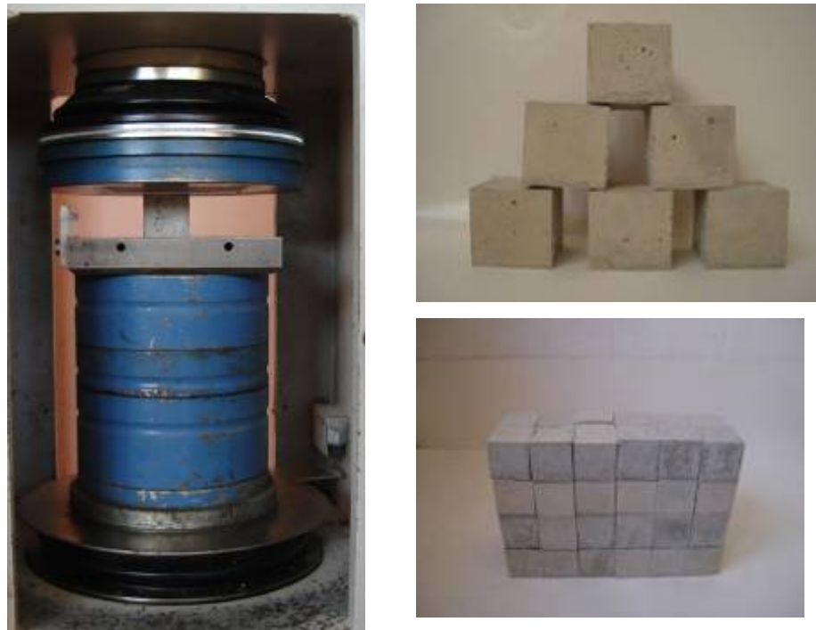
Figure 3.8 Compression testing machine and cubic samples
