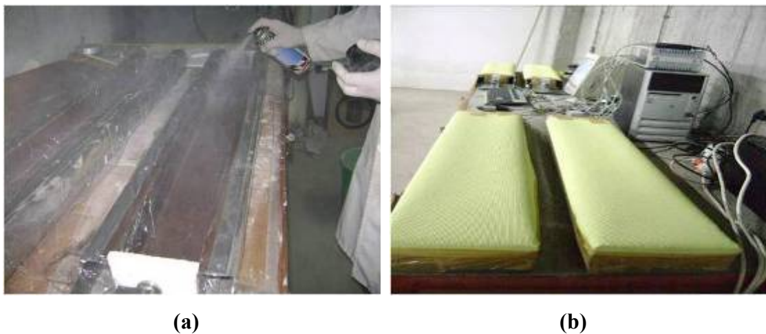
Figure 3.14 View of autogenous shrinkage test set-up a) during the preparation b) during the autogenous shrinkage test
