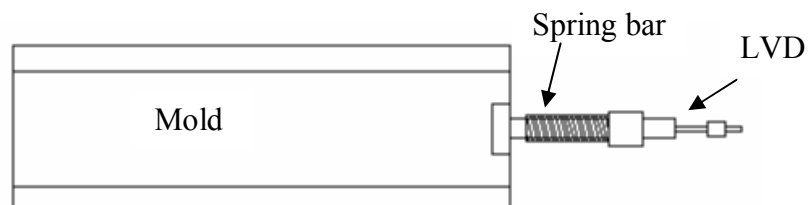
(c) Mold, LVDT and spring bar
