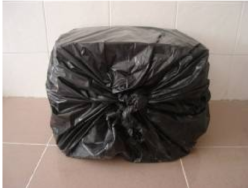
Figure 3.7 Moist curing of HES-ECC specimens after production
