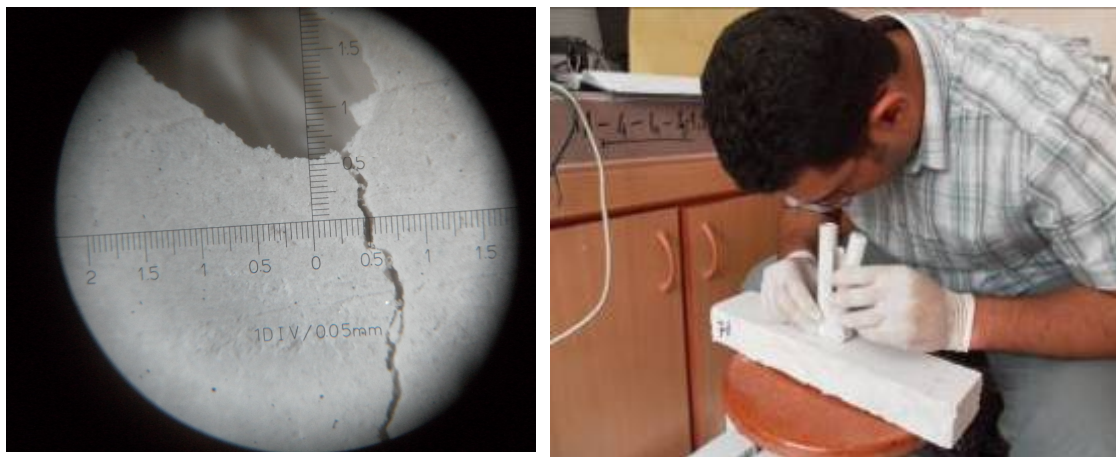
Figure 3.10 Controlling for crack widths of specimens after tested by four-point test
