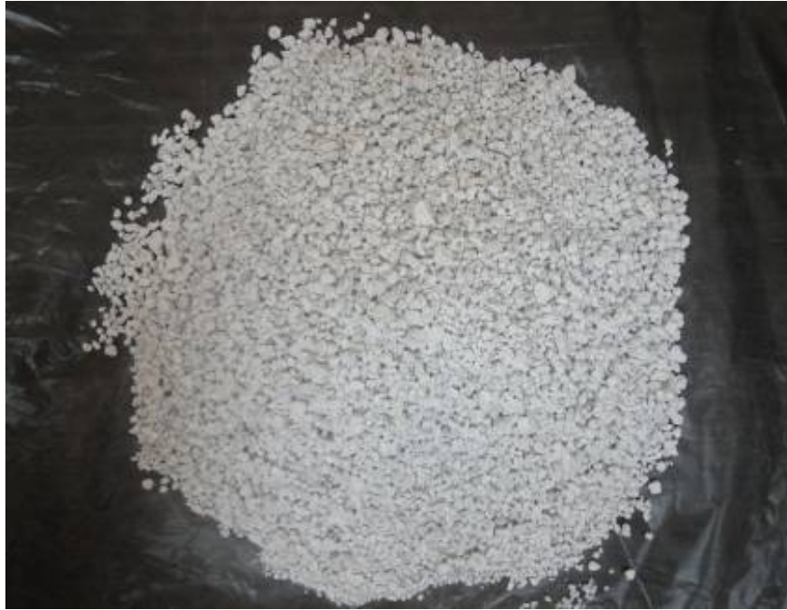
Figure 3.3 A view of expanded coarse perlite (LWA)
