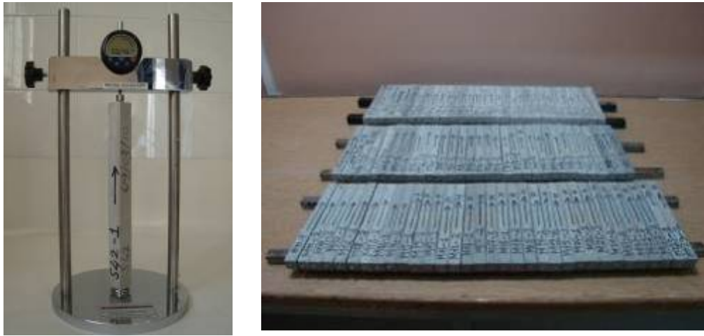
Figure 3.15 Drying shrinkage device and samples
