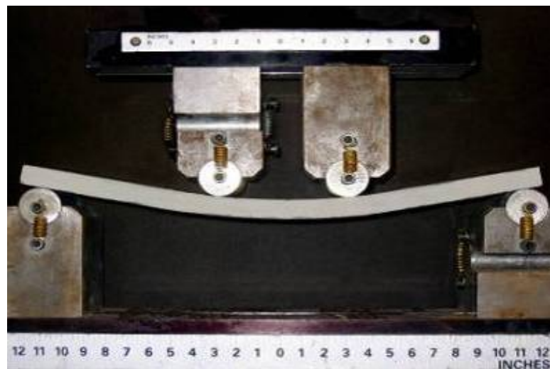
Figure 2.9 ECC's Behavioural Response against flexural loading
