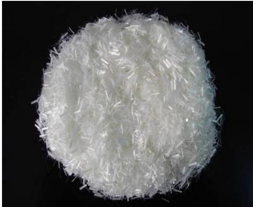
Figure 3.4 PVA fiber used in the production of ECC
