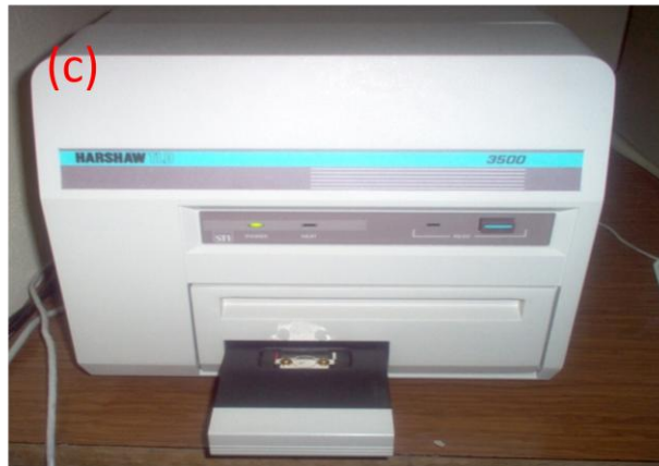
Figure 4.2 Experimental equipments (a) ^{90}\text{Sr} - ^{90}\text{Y} \beta -source (b) 9010 Optical Dating System (c) Harshaw TLD System 3500.
