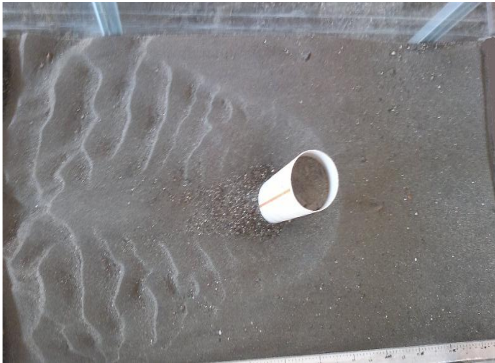
Figure 4.30 Experimental work shows pier for group 3 ( d=11.1\text{cm} )
