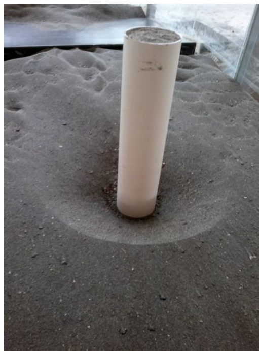
Figure 4.17 Equilibrium scour depth for Group 2 tests ( d=7.5\text{cm} )
