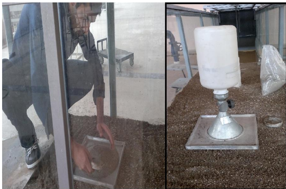
Figure 3.5 Sand specific gravity field test
