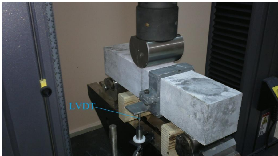
Figure 3.8 Photographic views of notched beam specimen
