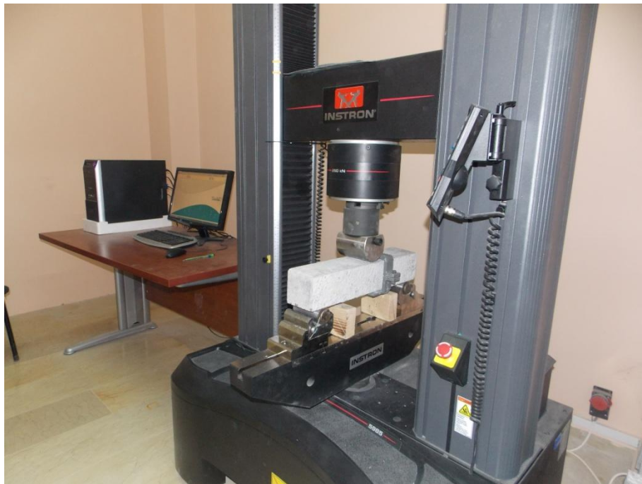
Figure 3.6 Photographic view of universal testing device and three point flexural testing fixture
