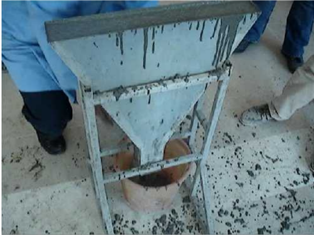
Figure 3.3 Photographic view of V-funnel flow time measurement
