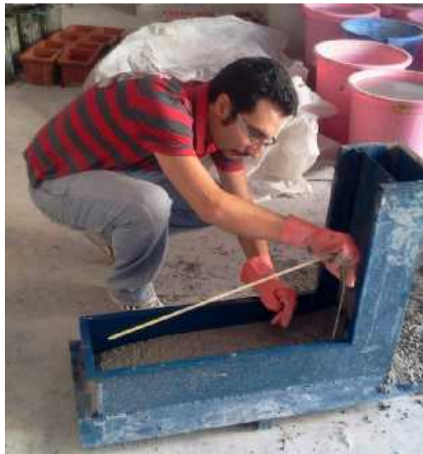
Figure 3.4 Photographic view of L-box apparatus and testing procedure
