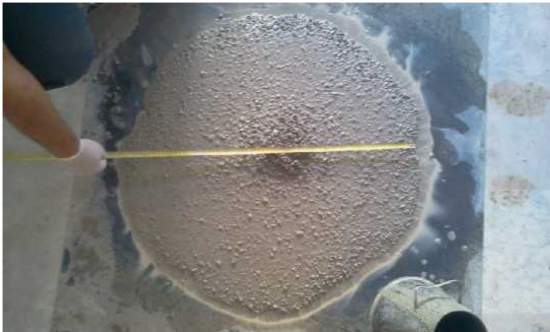
Figure 3.2 Photographic demonstration of measurement of slump flow diameter
