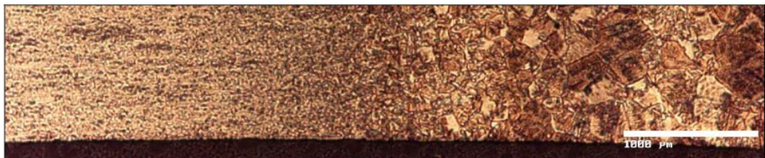
Figure 3.5 Base plates and Heat Affected Zone (HAZ) [34].
