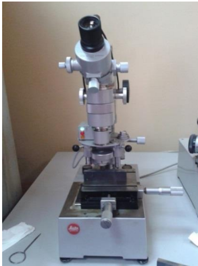
Figure 4.3 Micro-hardness testing (Vickers Hardness HV).
