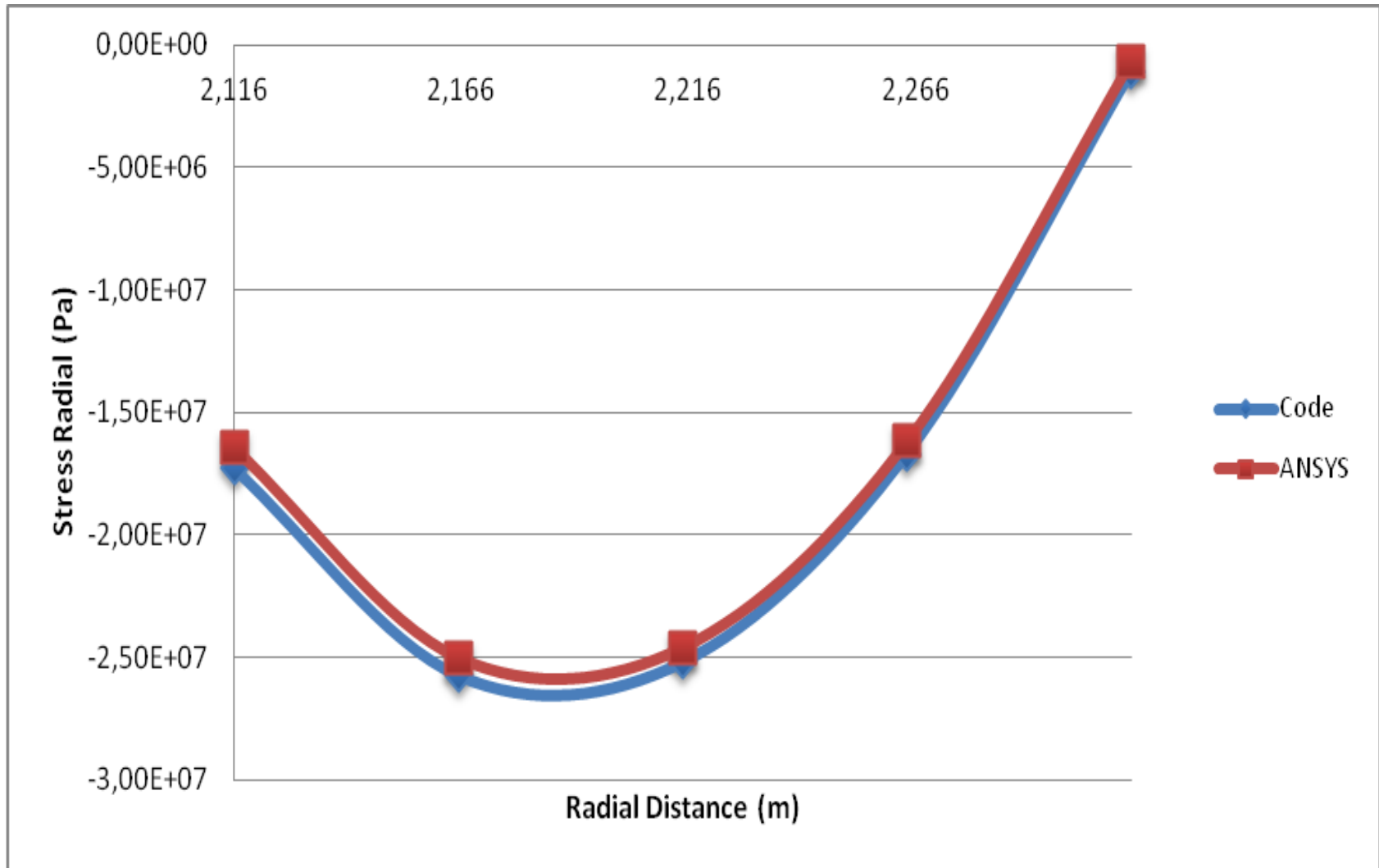
Figure 6.12. Radial stresses through the radial distance by ANSYS and our code at y=0 cross-section.
