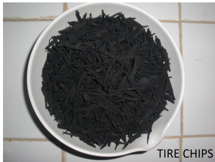
Figure 5.2. Waste tire rubber replaced with fine aggregate.
