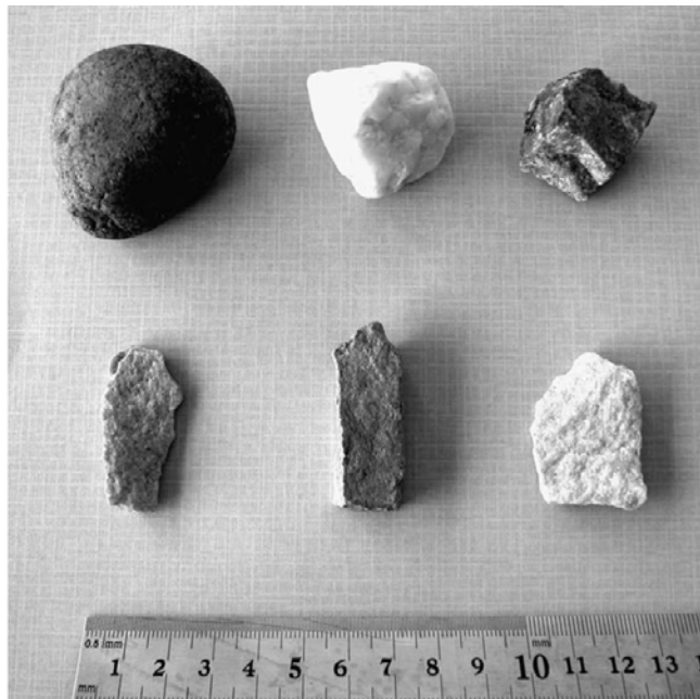
Figure 3.6. Illustrations of particle shapes. Shapes are, clockwise from top left: Rounded, Irregular, Angular, Flaky, Elongated, Flaky and Elongated. [46]
