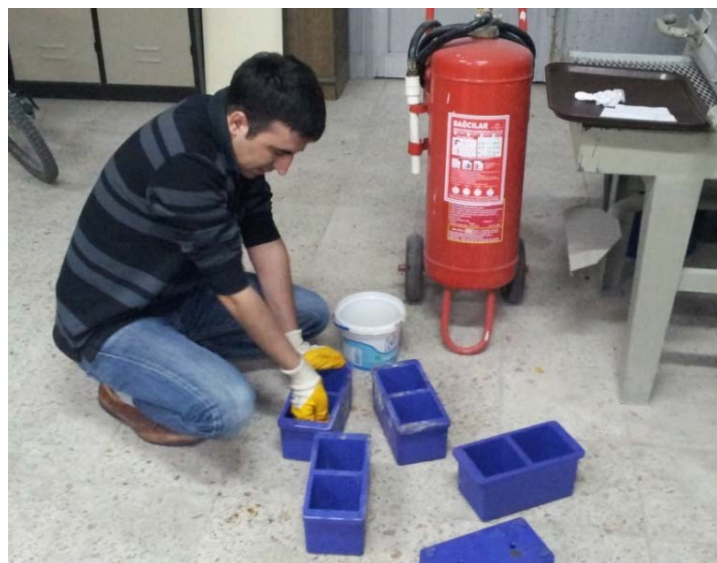
Figure 5.4. Cubic samples 100 x 100 x 100 mm
