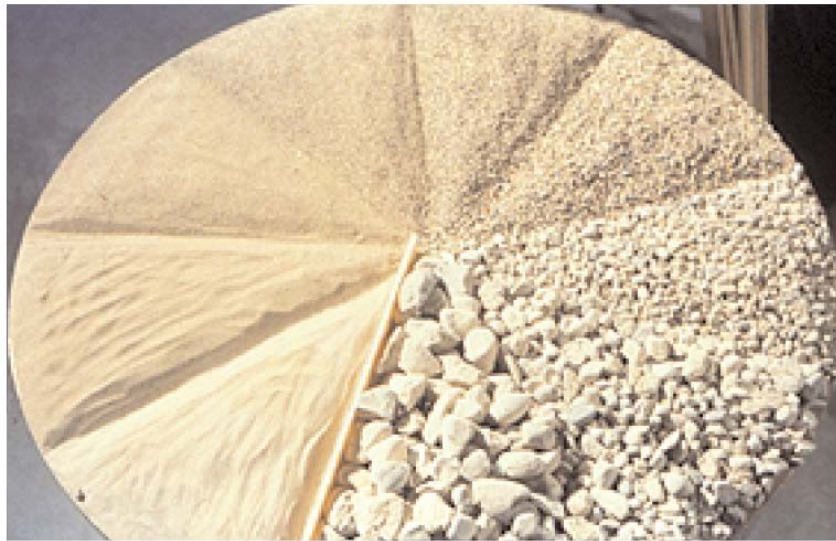
Figure 3.8. Range of particle sizes found in aggregate for use in concrete. [40]
