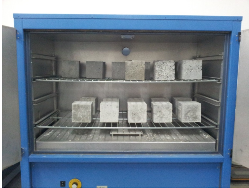
Figure 5.8. Hardened concrete samples in oven
