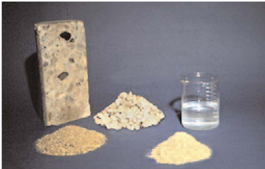
Figure 3.1. Concrete components are combined to form concrete [40]
