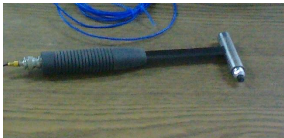
Figure 4.8 PCB 086C03 modal impact hammer
