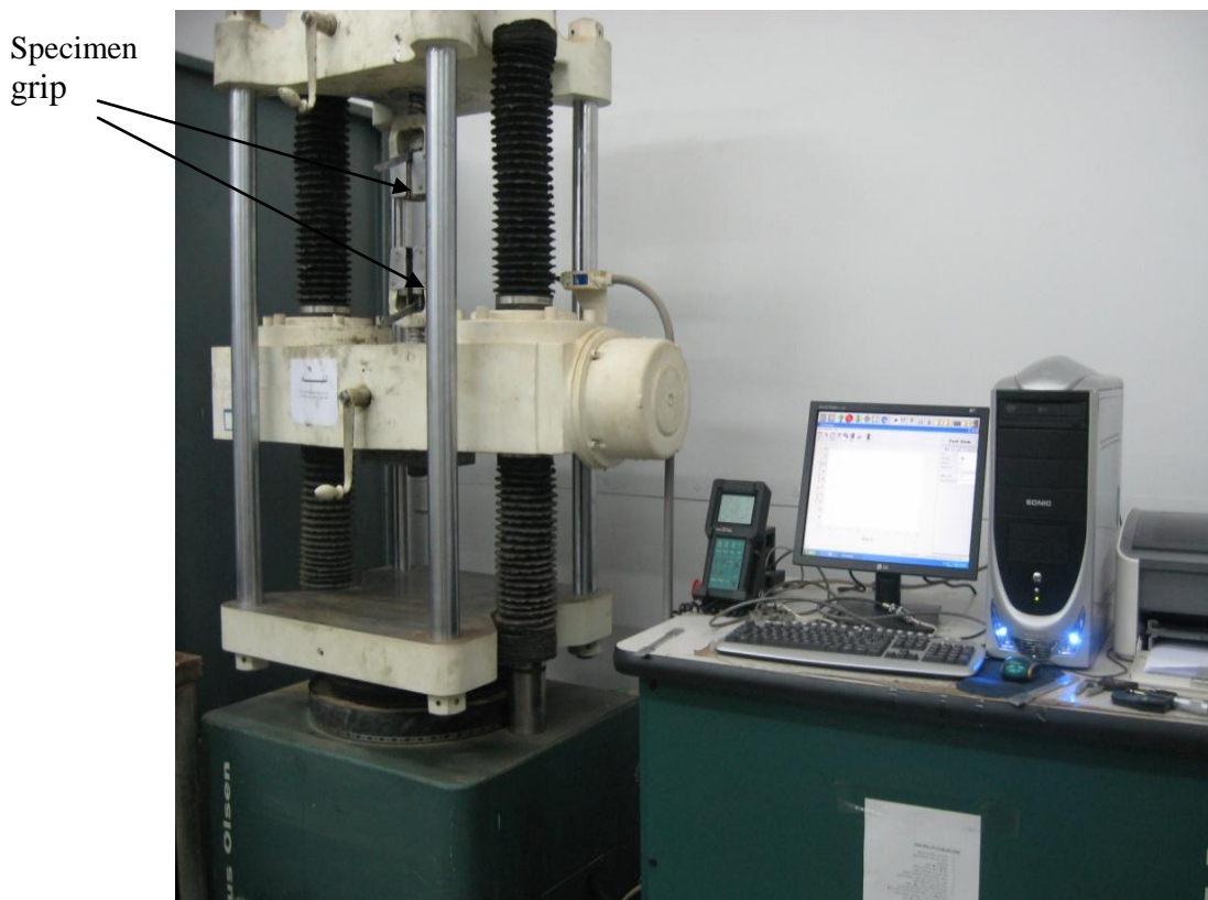
Figure 3.6 Tinius Olsen universal tensile testing machine in Central Organization for Standardization & Quality Control.
