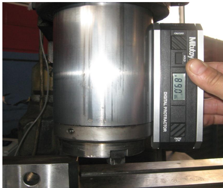
Figure 3.3 The digital scale used for rotating the head of the vertical milling machine to satisfy the required tilt angle
