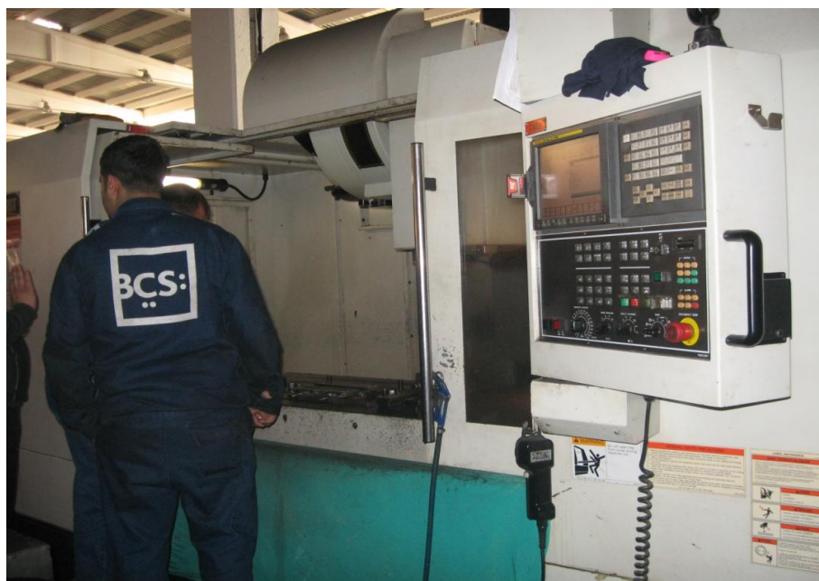
Figure 3.2 The milling machine utilized for friction stir welding (FANUC Series 21-MB)
