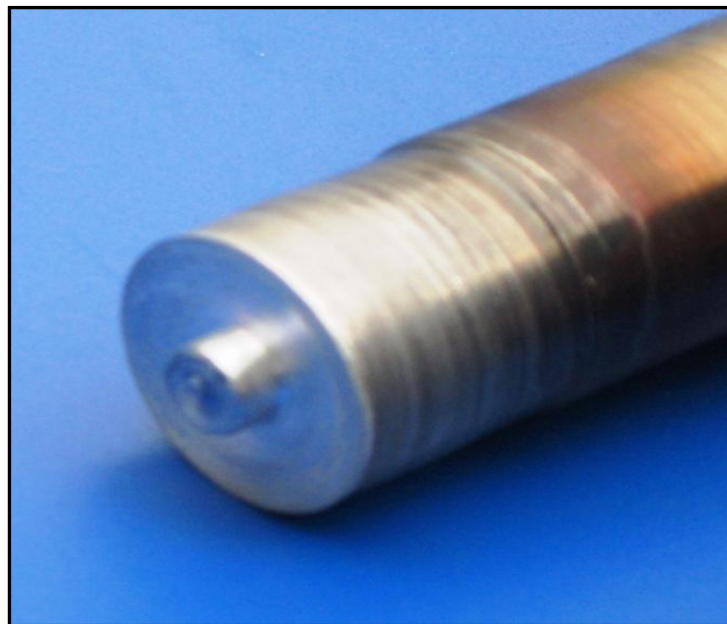
Figure 3.1 (a) FSW tool used in the current study
