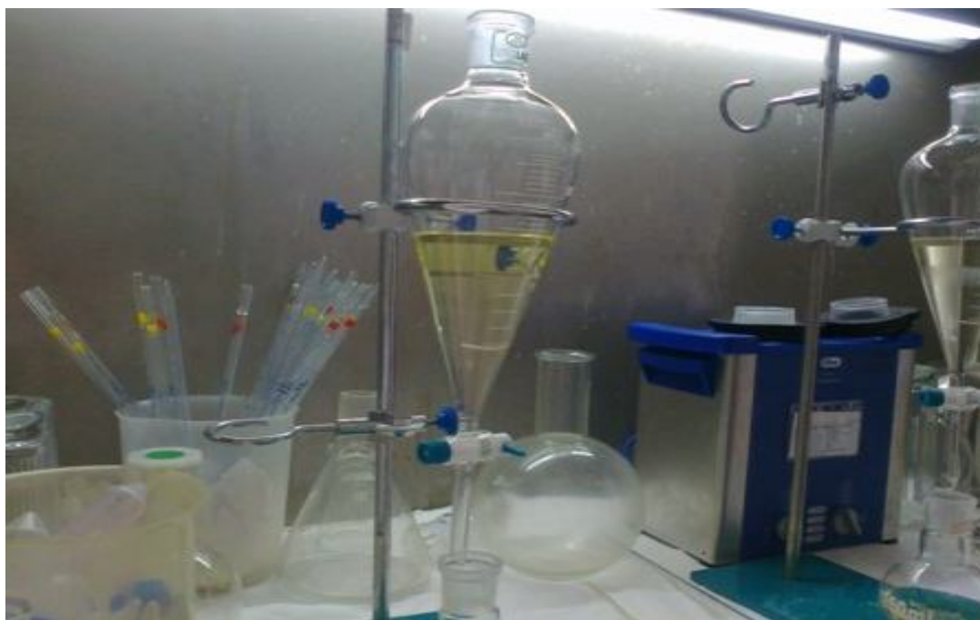
Figure 2.1 Phase separation in separating funnel
