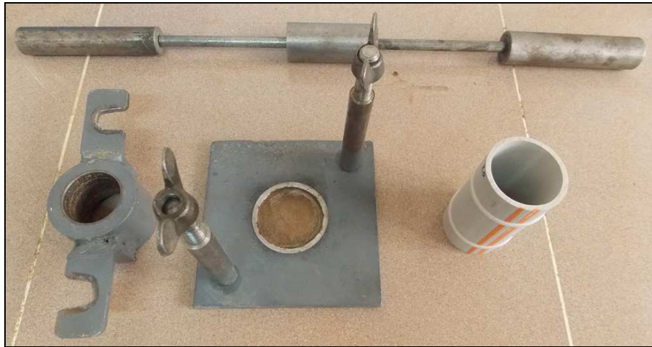
Figure 3.8 Equipments of the UCS test used during the experimental work
