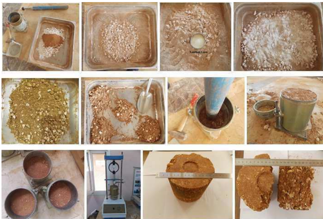
Figure 3.5 Pictures of testing process for CBR
