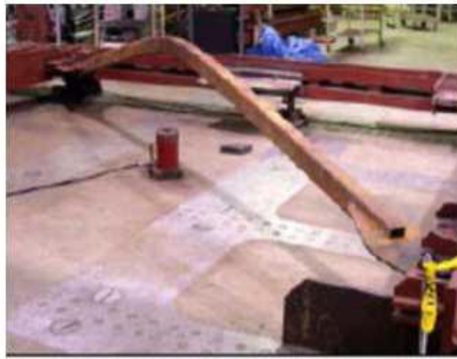
Traditional brace, buckled in compression
