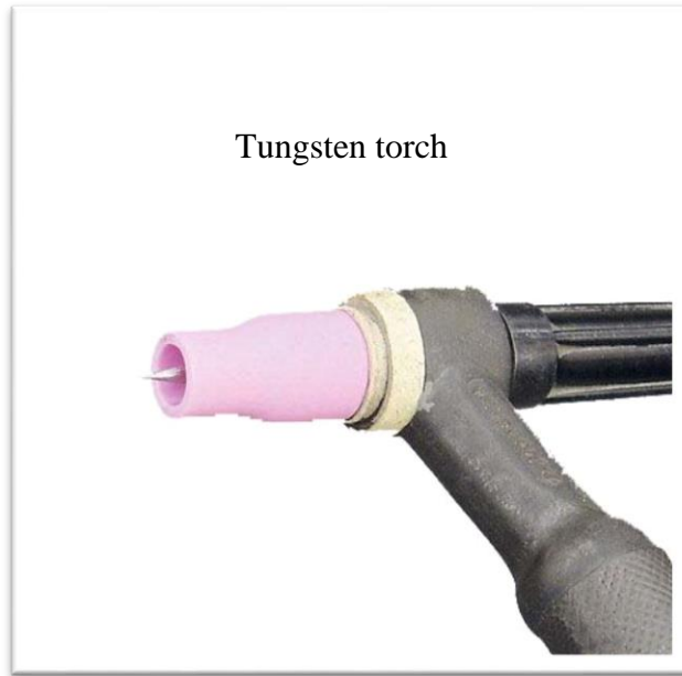
Figure 4.5 Tungsten Torch used in Welding Stainless Steel
