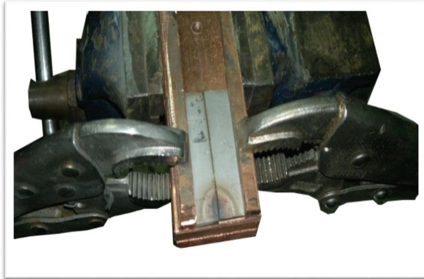
Figure 4.6 Fixing Stainless Steel to Avoid Distortion
