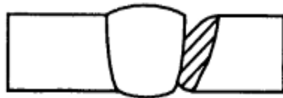
(c) (HAZ) corrosion type
