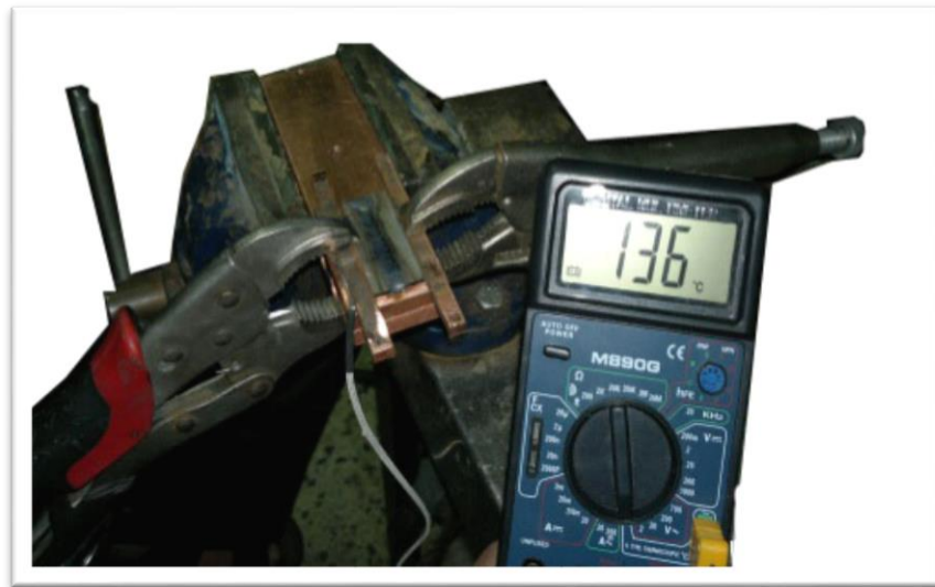
Figure 4.8 Temperature Measured by a Thermocouple.
