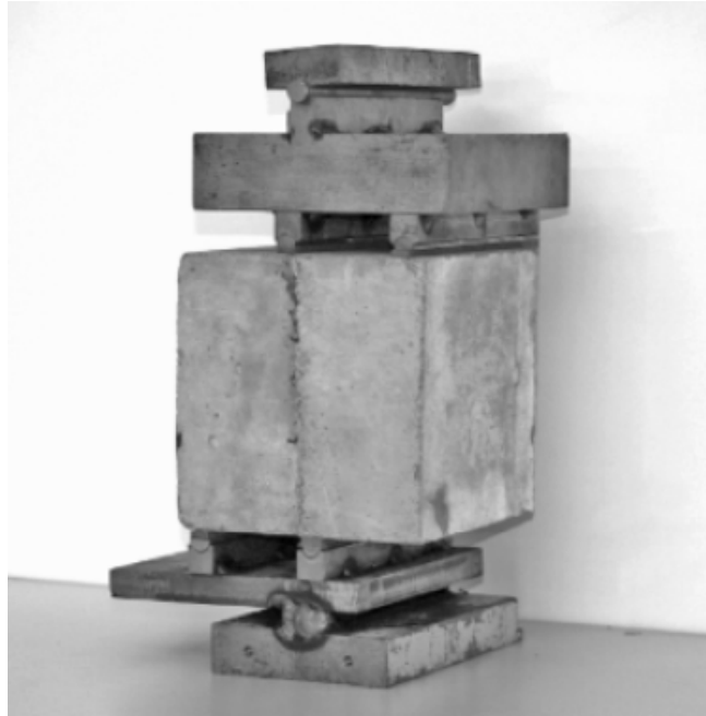
Figure 2.7 Photograph of interface shear bond test method used for short-term bond strength evaluation (Beushausen and Alexander, 2008)
