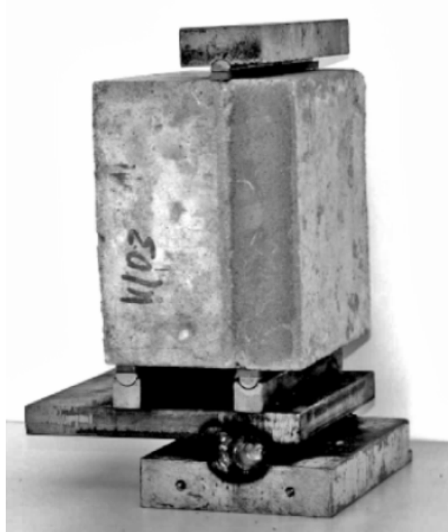
Figure 2.9 Photograph of interface shear bond test method, guillotine test (Beushausen and Alexander, 2008)
