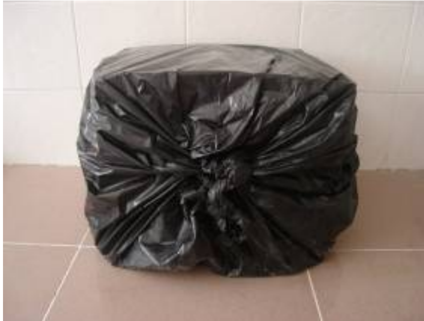
Figure 3.4 Moist curing of specimens to be used in mechanical property characterization after production
