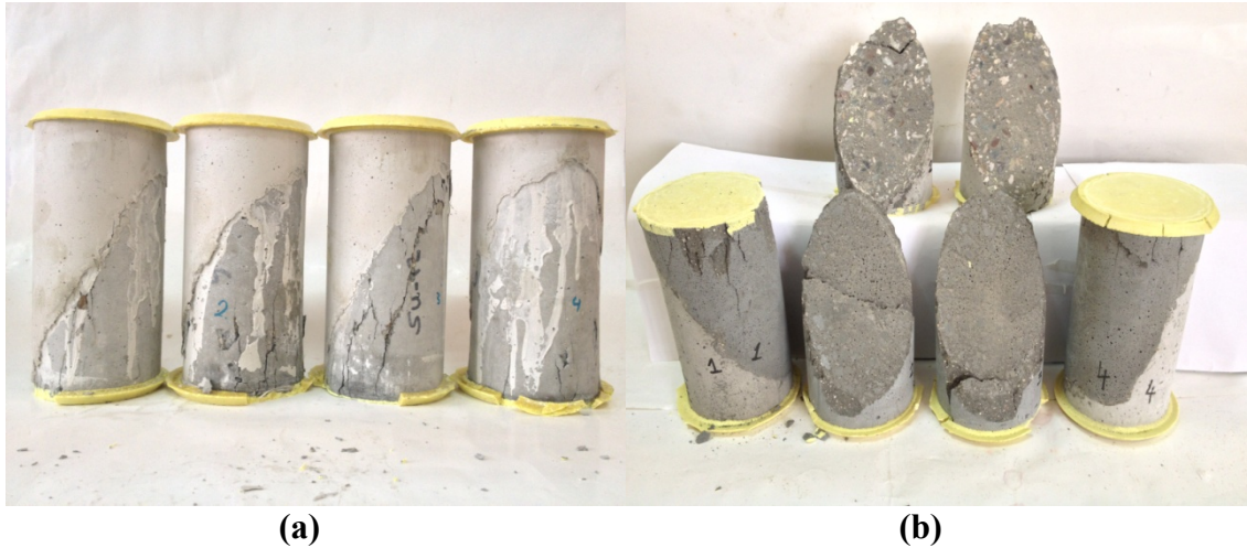
Figure 3.12 Failure modes of HES-ECC and REPM specimens at the end of 28 days as a result of slant shear tests
