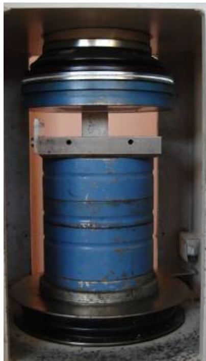
Figure 3.5 Compression testing machine and cubic samples
