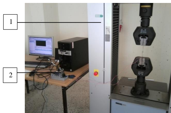
Figure 4.9 Test set-up (1) Shimadzu AG-X series testing machine, (2) Ni-9237 data acquisition card
