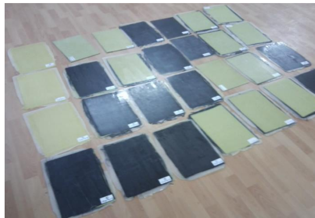
Figure 4.5 Example of produced symmetrical hybrid plates.
