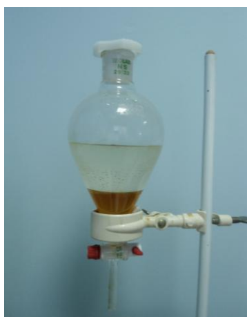
Figure 3.1. Oil extraction by separating funnel
