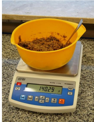
Figure 3.20. Biopolymer – sand mixture under preparation.
