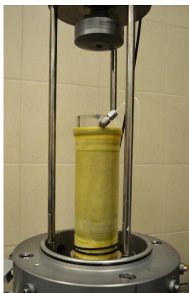
Figure 3.21. Prepared sample ready for triaxial testing.
