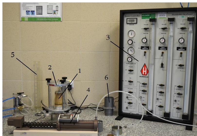
Figure 3.12. Permeability apparatus: 1- specimen; 2- triaxial cell; 3- cell pressure controller; 4- pore water controller; 5- out flow cylinder; 6- sample mould.
