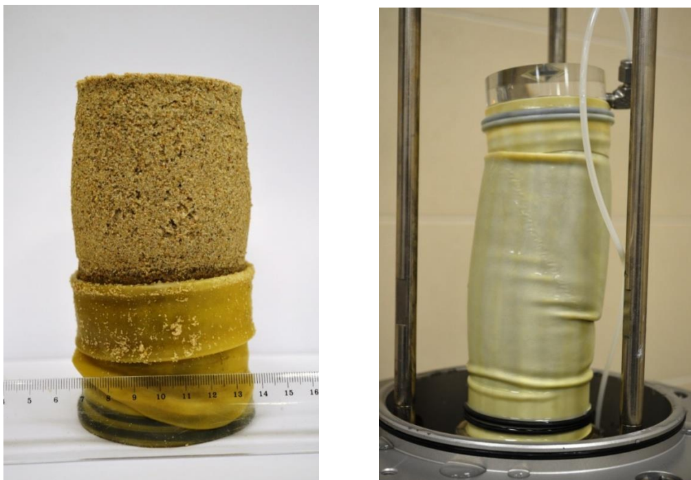
Figure 4.34. Samples after testing.
