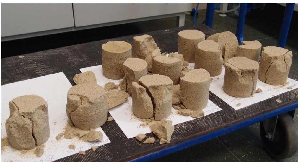
Figure 4.38. Samples after UCS test.
