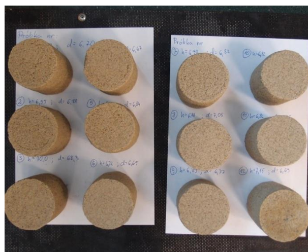
Figure 3.23. Solid sand-xanthan gum samples (a).
