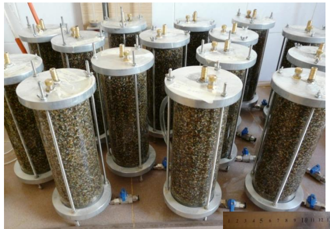
Figure. 3.9. Samples in the molds while curing [8.0 x 23.6 cm].
