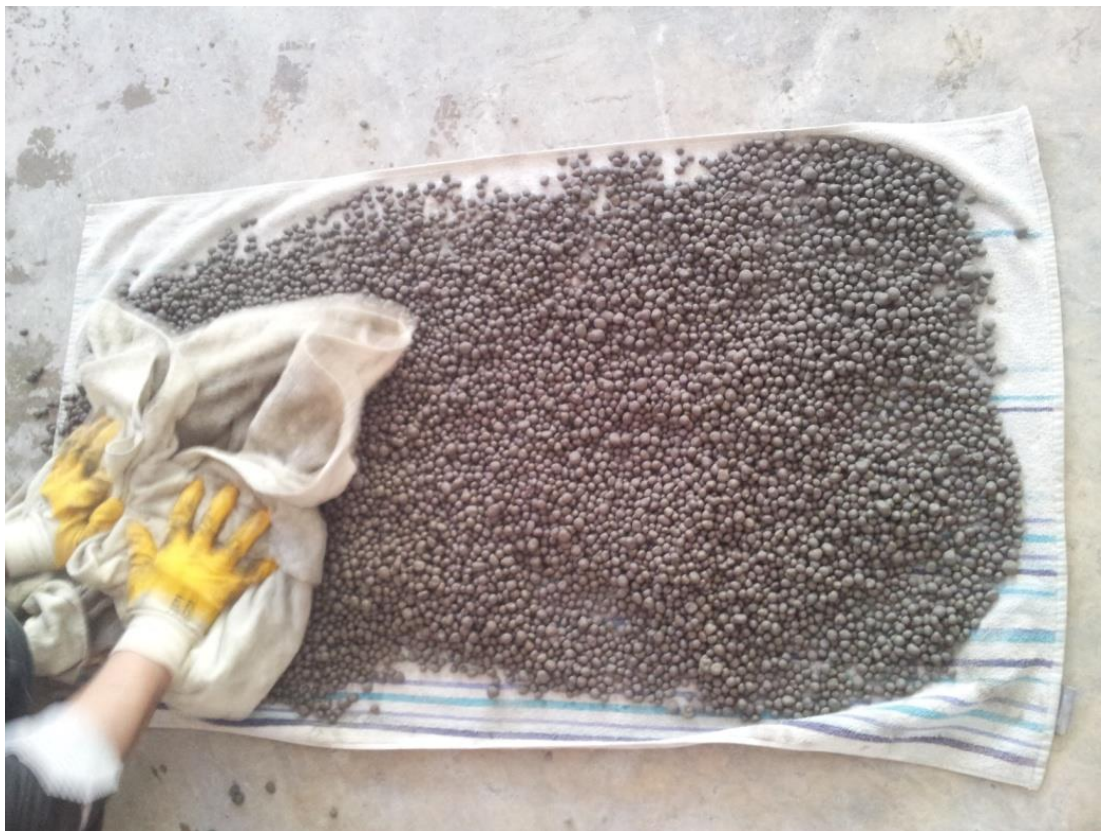
Figure 3.6 LWAs in SSD condition
