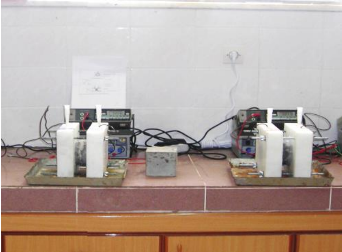
Figure 3.20 Photographic view of the RCPT test set up
