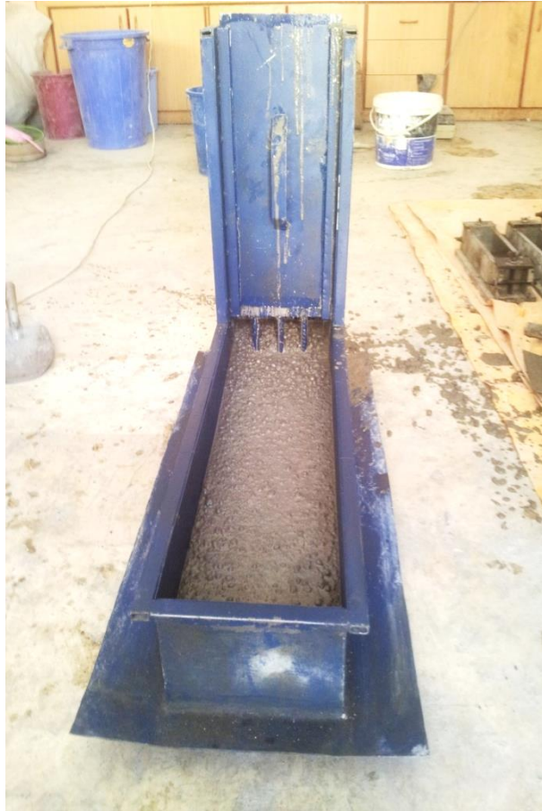
Figure 3.9 Photographic views of the L-box apparatus and test procedure
