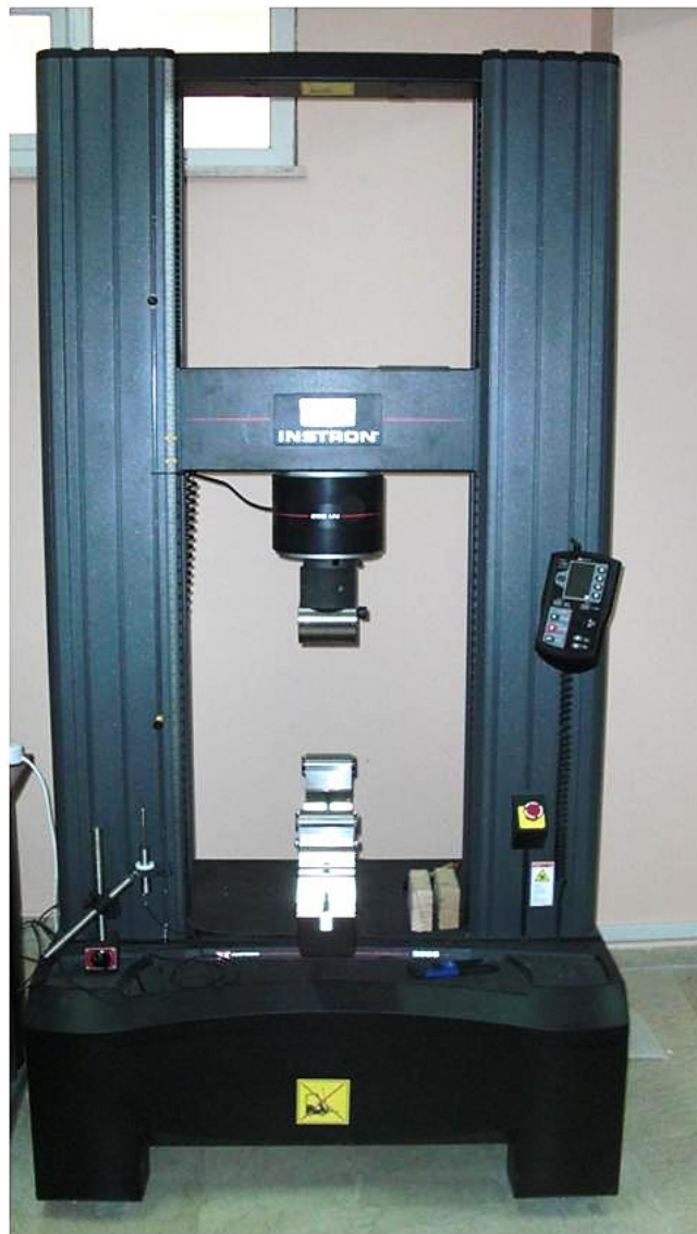
Figure 3.11 Photographic view of universal testing devices and three point flexural testing fixture
