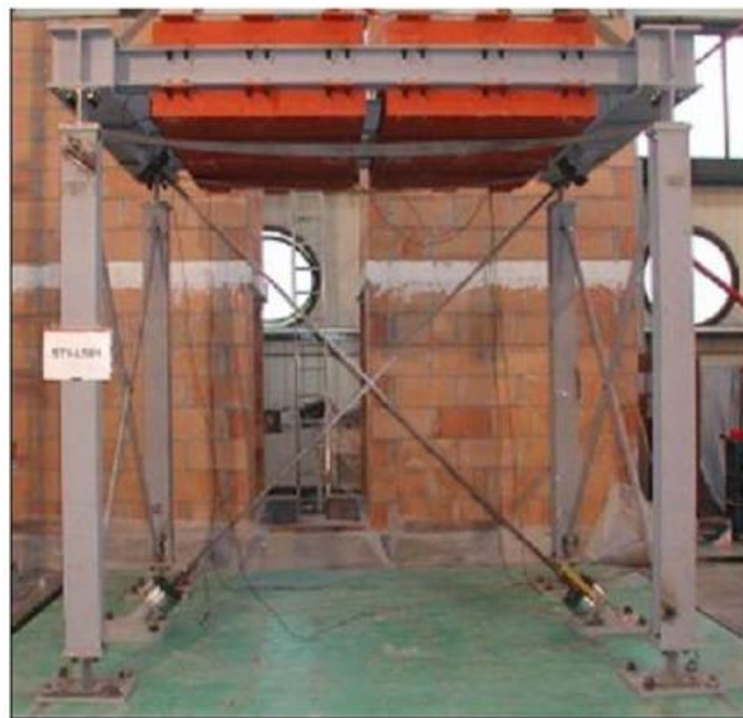
Figure 2.7 View of test frame on shake table prior to testing (Broderick et al., 2008)
