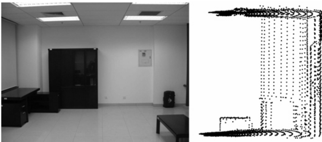
Figure2.2 Real Environment and 3D point cloud
