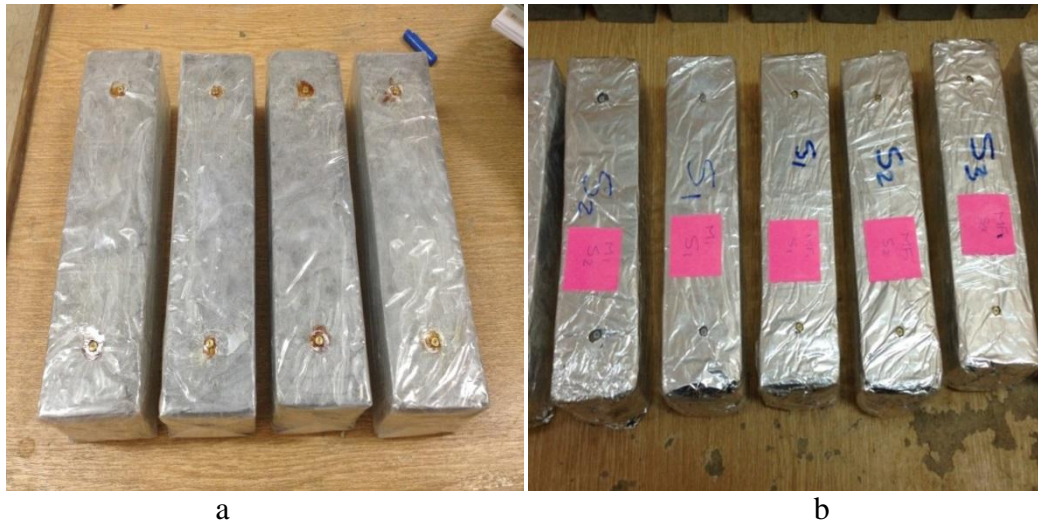
Figure 3.7.a-) Specimens sealed with two layers of plastic sheets. b-) After plastic sheets specimens sealed with a layer of aluminum foil
