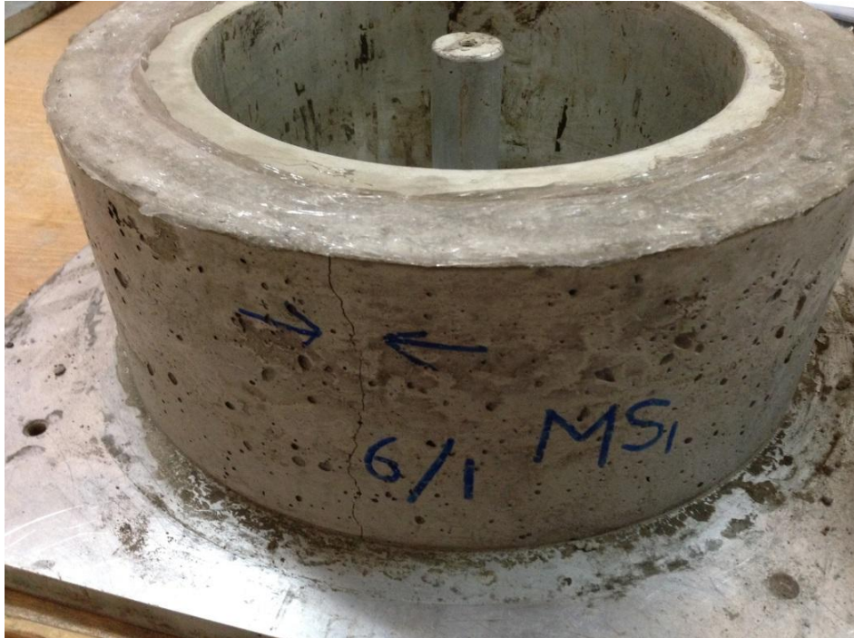
Figure 3.16 Photographic view of a cracked ring specimen
