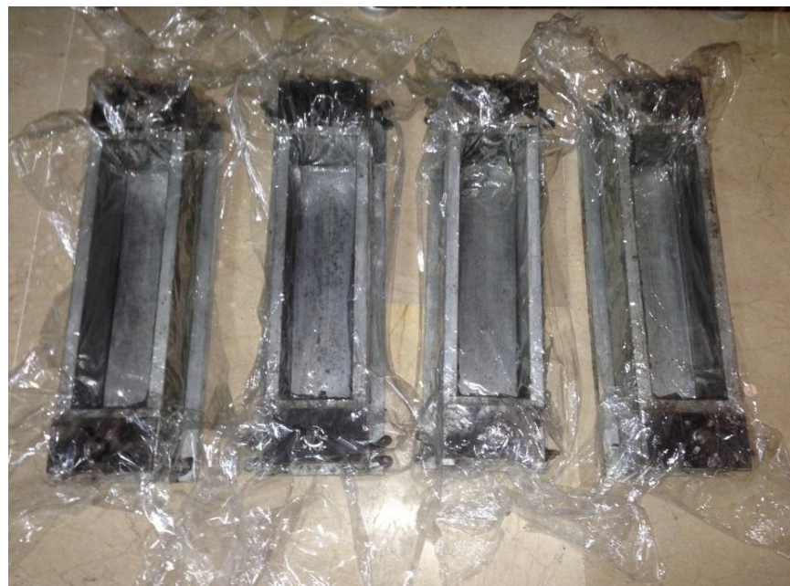
Figure 3.6 Plastic sheets inside the mold before the casting
