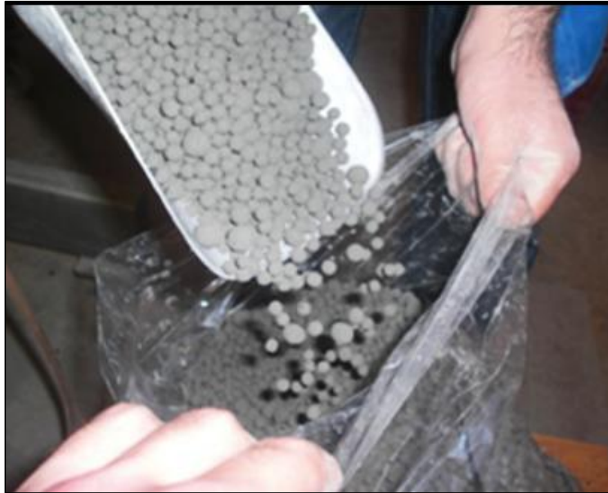
Figure 3.2 Artificial aggregate self-curing process
