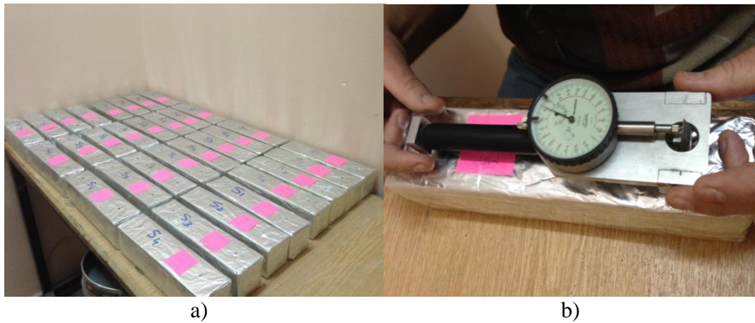
Figure 3.12: a) Autogenous test specimens. b) Test apparatus
