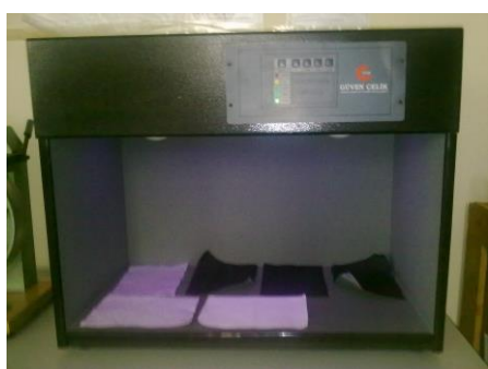
Figure 5.9. UV resistance tester with samples in it
