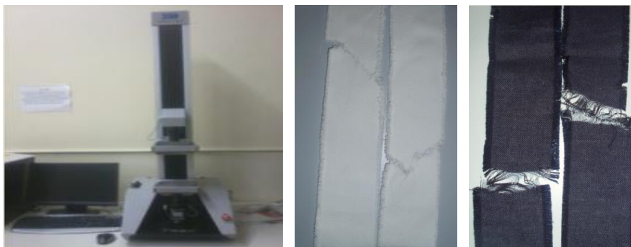
Figure 5.6. Breaking strength tester and final situations of samples
