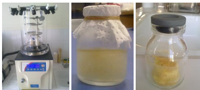
Figure 5.4. Lyophilization machine and Aloe vera gel before and after process
