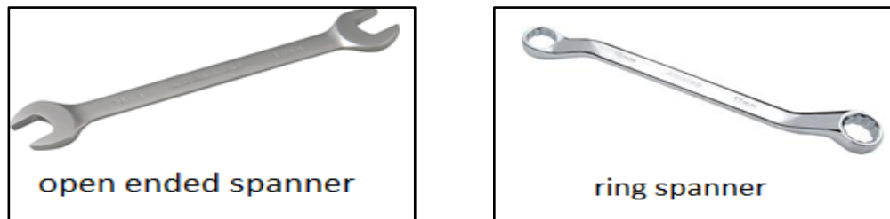
Figure 1.4 General types of spanners
