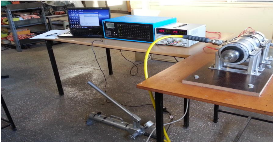
Figure 4.11 General view of all components of hydraulic tensioning test system
