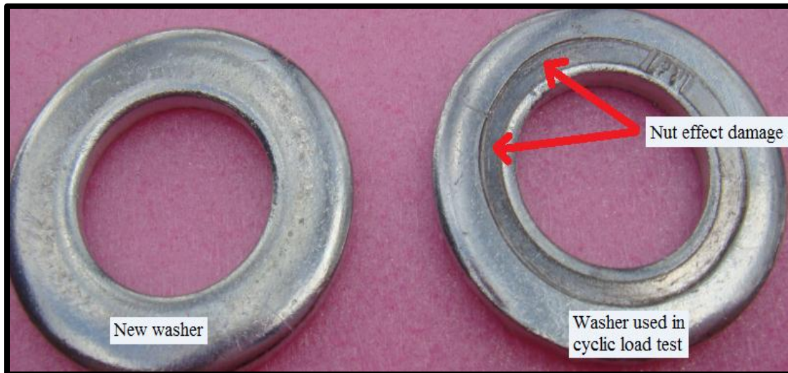
Figure 5.17 Conventional torque tightening and cyclic load effect on washer surface
