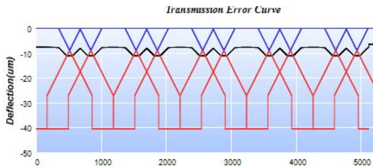
Figure 6.16 TE curve for 7620 N design load from Software
