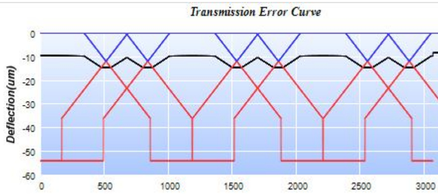
Figure 6.40 TE curve for 10160 N design load from software
