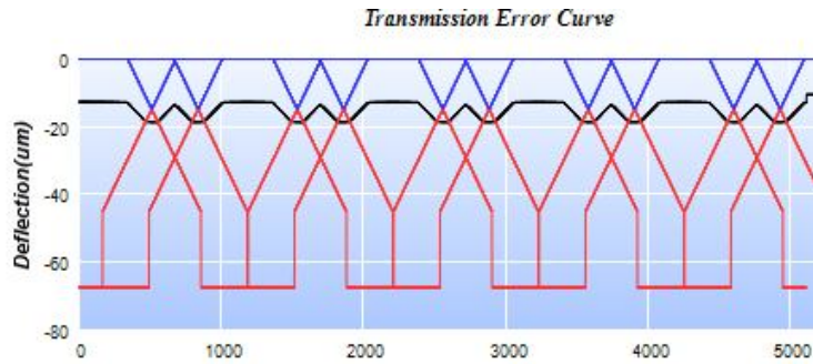
Figure 6.24 TE curve for 12700 N design load from software
