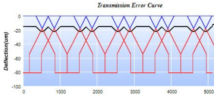
Figure 6.28 TE curve for 15240 N design load from Software
