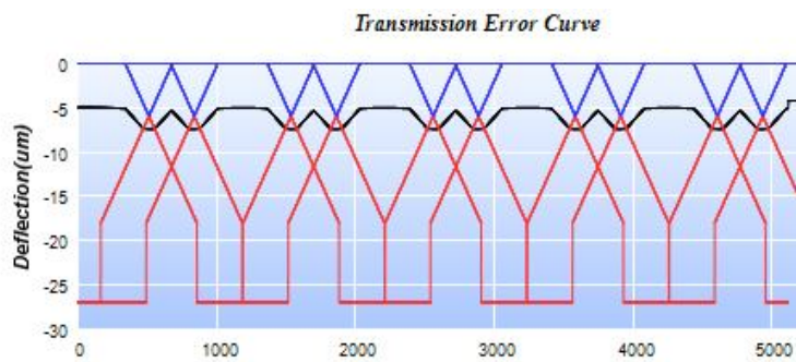
Figure 6.12 TE curve for 5080 N design load from Software
