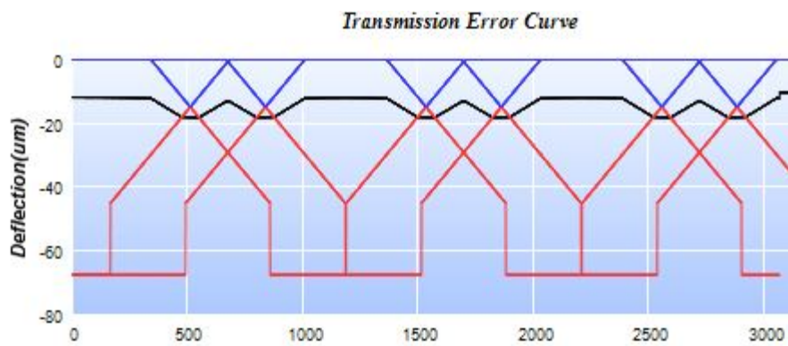
Figure 6.44 TE curve for 12700 N design load from software
