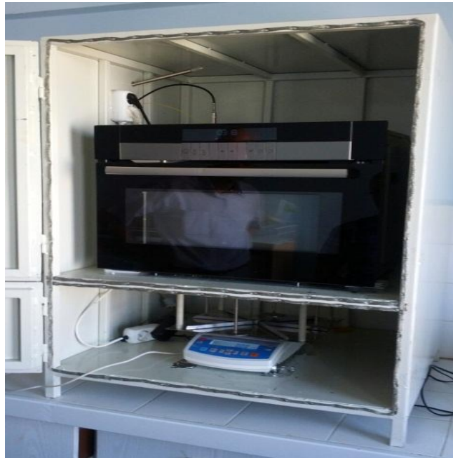
Figure 3.2 Air - circulating microwave oven used in drying of tomato
