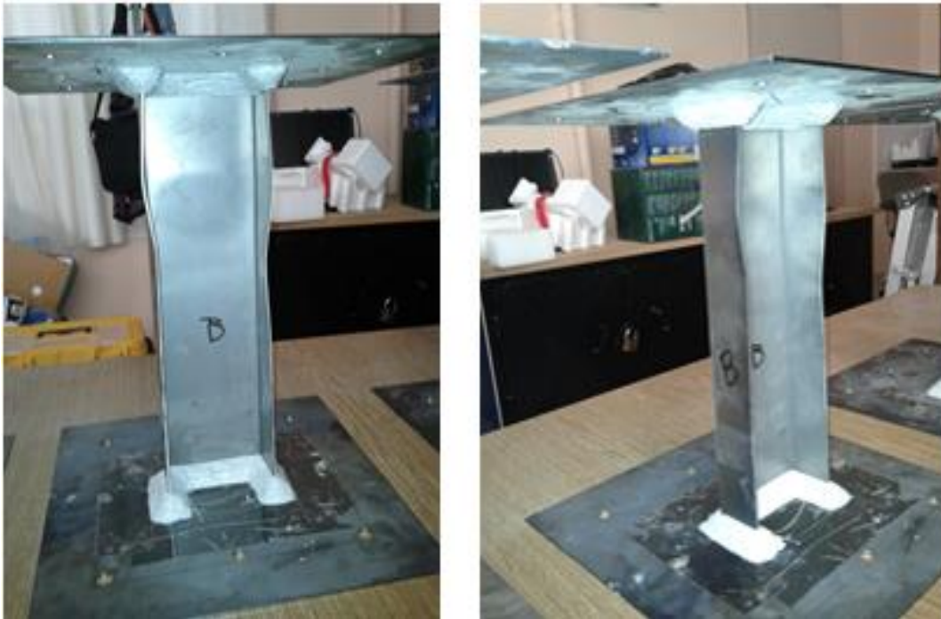
Figure 5.18 Failure modes of test specimens UC 93-41
