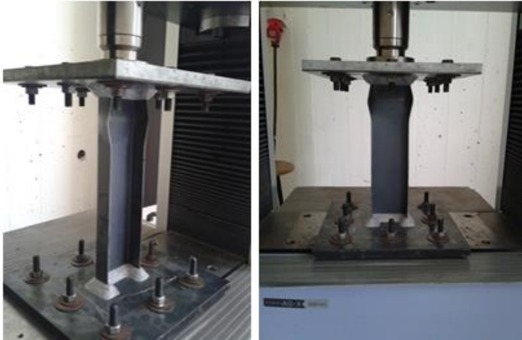
Figure 5.16 Failure modes of test specimens UC 82-31
