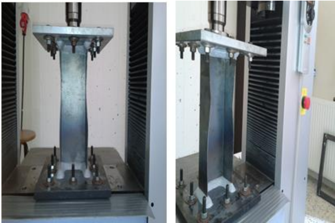
Figure 5.24 Failure modes of test specimens UC 123-71
