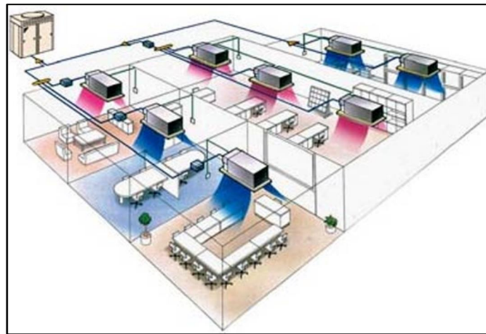
Figure 3.10 Heat recovery VRF system
