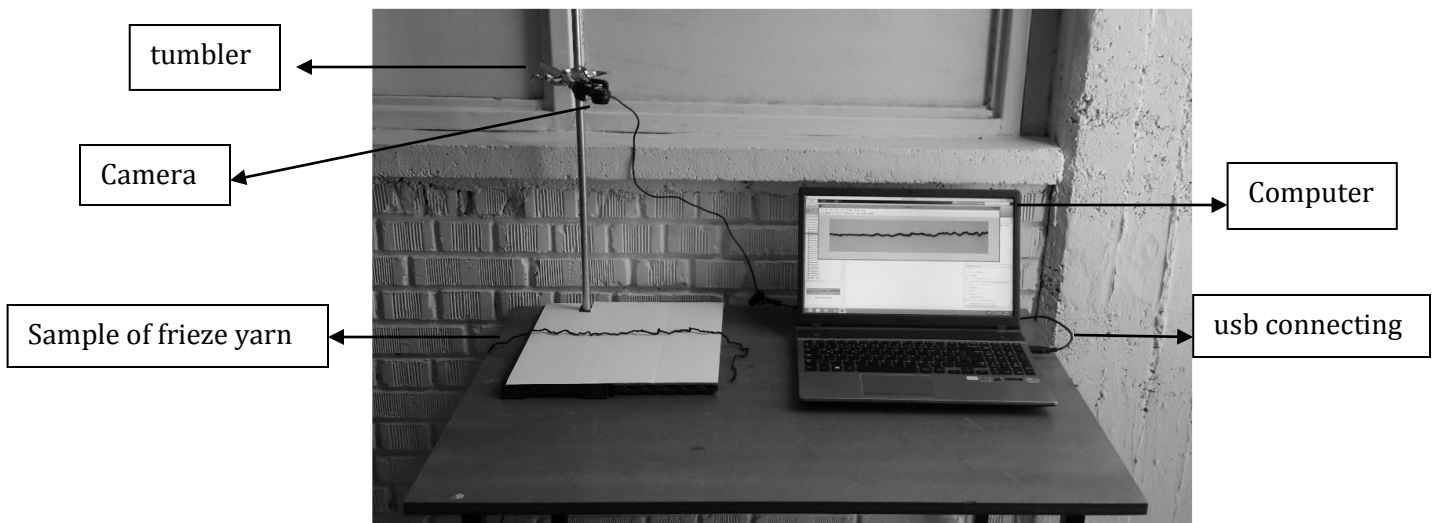
Figure 4.1 A simple computer vision system to count the crimp on the yarn
