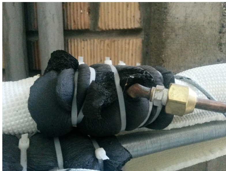
Figure 5.9 Insulating of contact point between pipe and thermocouple
