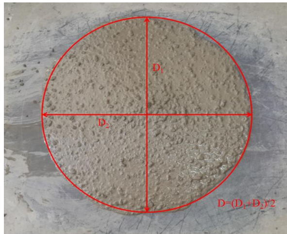
Figure 4.1 Measurement of slump flow diameter for SCCs (Control mixture)
